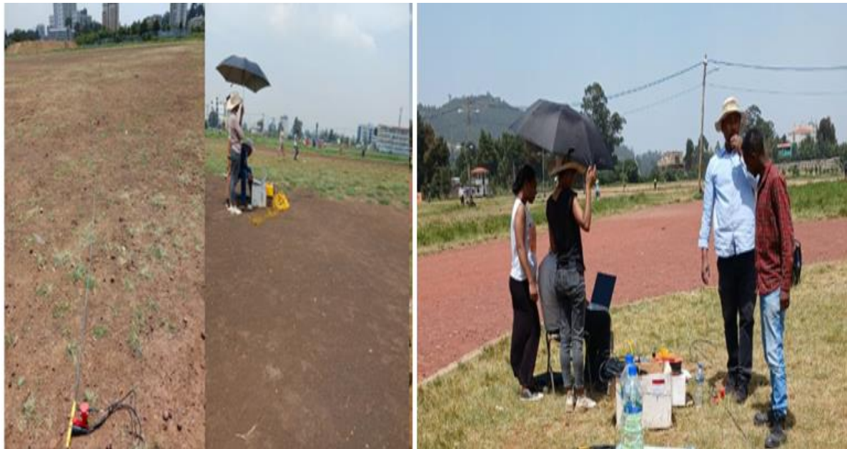
Figure 3.16: Active and passive MASW data acquisition field campaign at Jan-Meda
