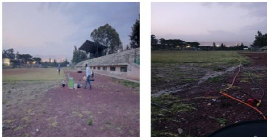
Figure 3.15: MASW data acquisition at bole community school
