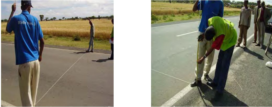
Fig. 3.4 Measuring superelevation on horizontal curve
