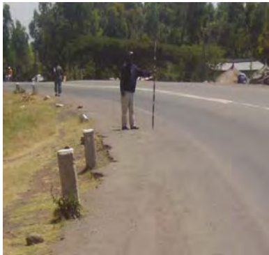
Fig. 3.2 Speed measuring and locating the center of horizontal curves
