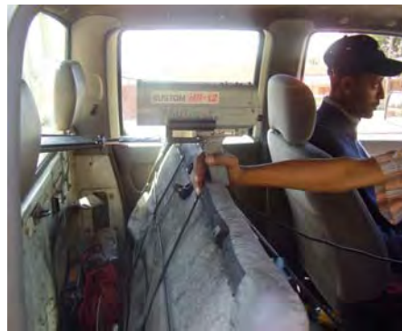
Fig. 3.2 Speed measuring and locating the center of horizontal curves
