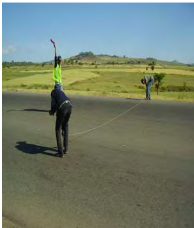
Fig. 3.3. Measuring pavement width and grade on curve and tangent
