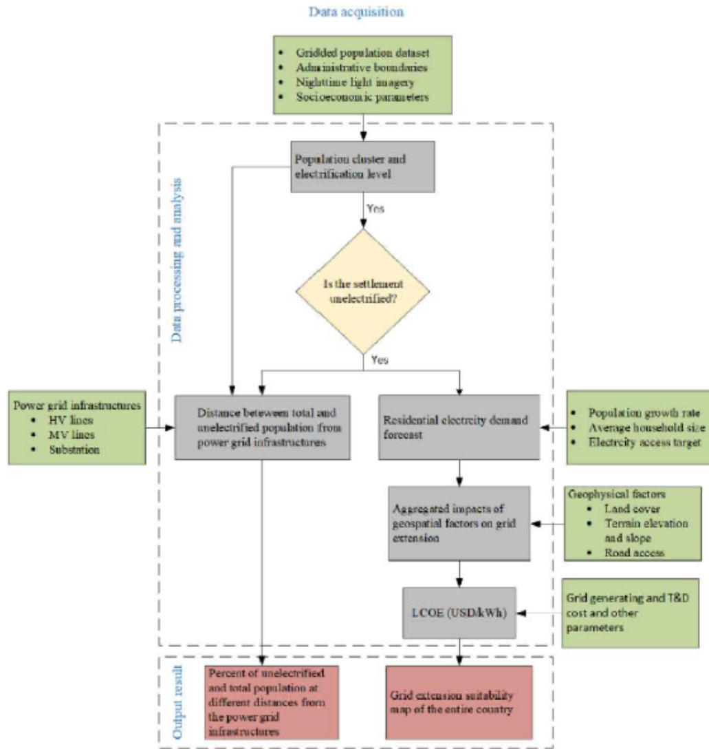
Fig. 1. Flowchart of methodological approach. Diagram color shows: olive green “input data”, gold and grey “data process” and red “results of the analysis”.
