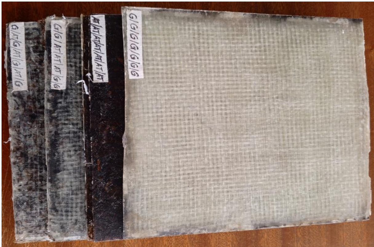
Figure 21 all fabricated composite panels
