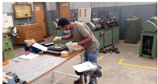
Figure 19 setup and hand lay-up fabrication of composite laminates
