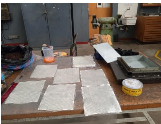
Figure 19 setup and hand lay-up fabrication of composite laminates
