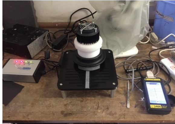
Figure 3-5 Irradiance measurement using UVC-LEDs
