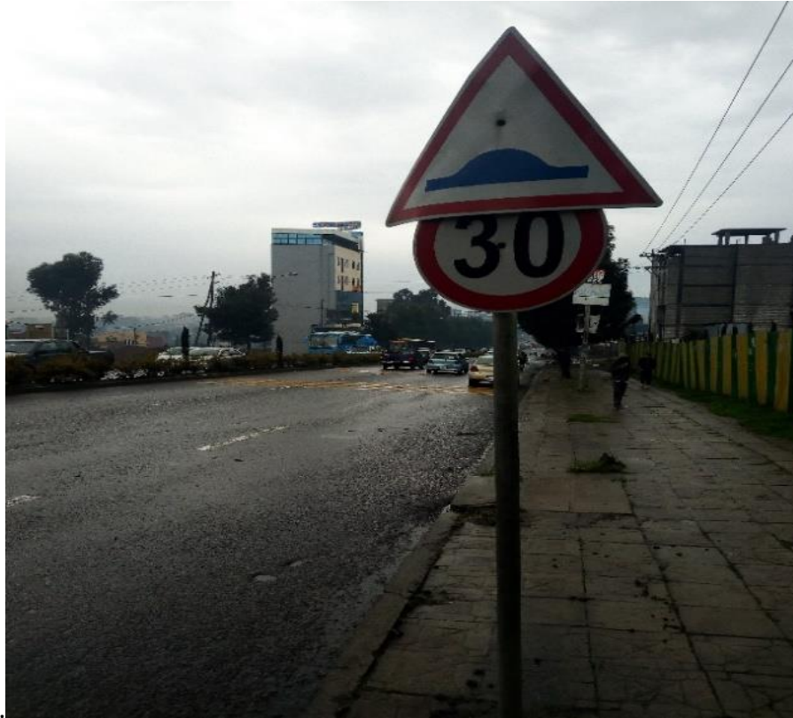
Figure 4- 16 Speed Hump Warning Sign
