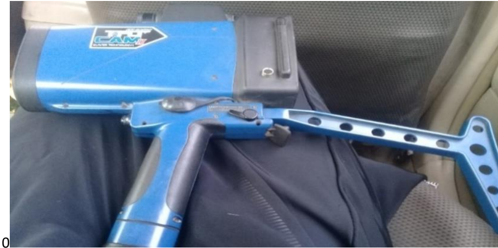
Figure 2- 13 a hand-held digital radar gun (Laser Technology)
