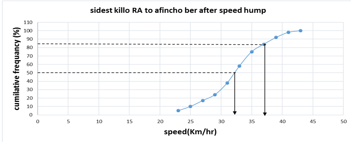
Figure G- 1 Cumulative frequency curve with 85th & 50th level marked by dotted lines after speed hump
