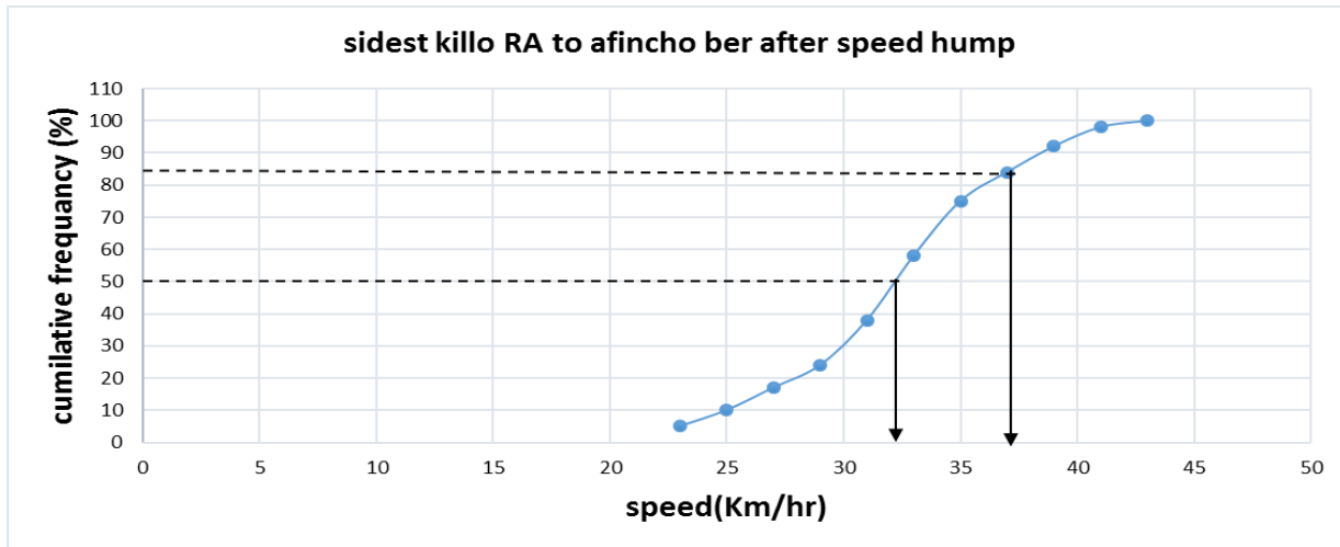
Figure 4- 31 Cumulative frequency curve with 85th & 50th level marked by dotted lines after speed hump
