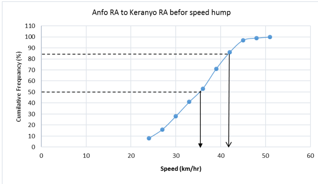
Figure E- 13 Cumulative frequency curve with 85 th & 50 th level marked by dotted lines before hump
