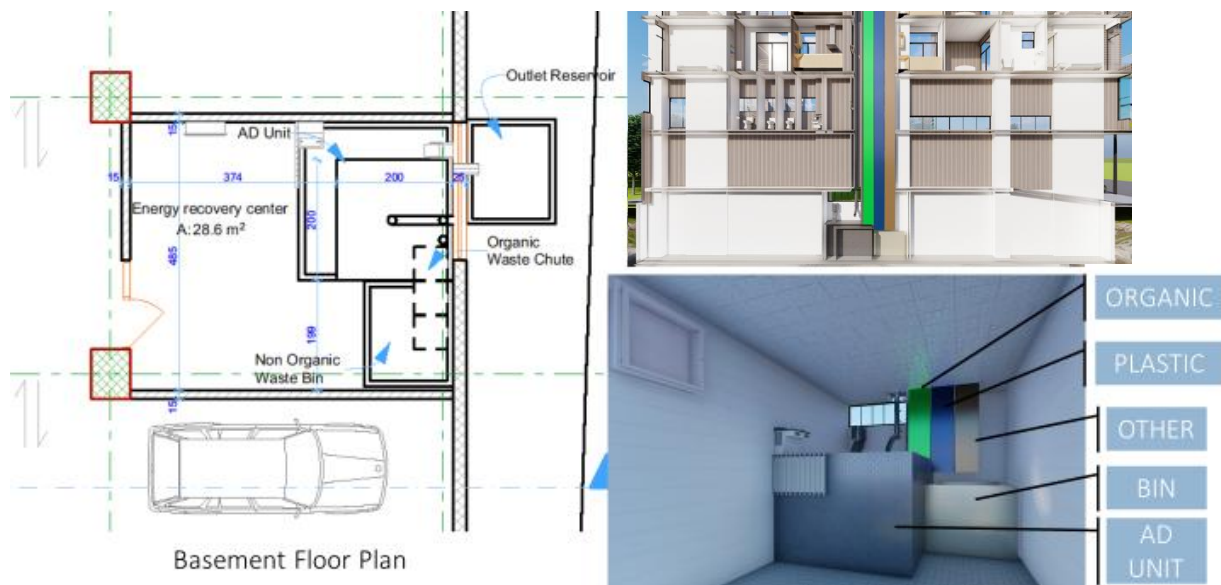
Figure 4.13. Schematic Layout of Anaerobic Digestion (AD) Integration in Basement
