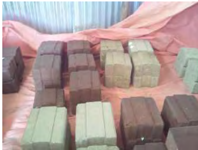
Photo 3.2 Curing of the blocks under cover produced in East-Horizon Consultant block production center.
