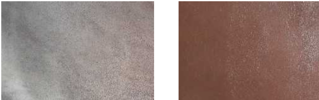
Fig4.17 a) Dyed crust leather ready for cationic finishing and b) Cationic finished leather
