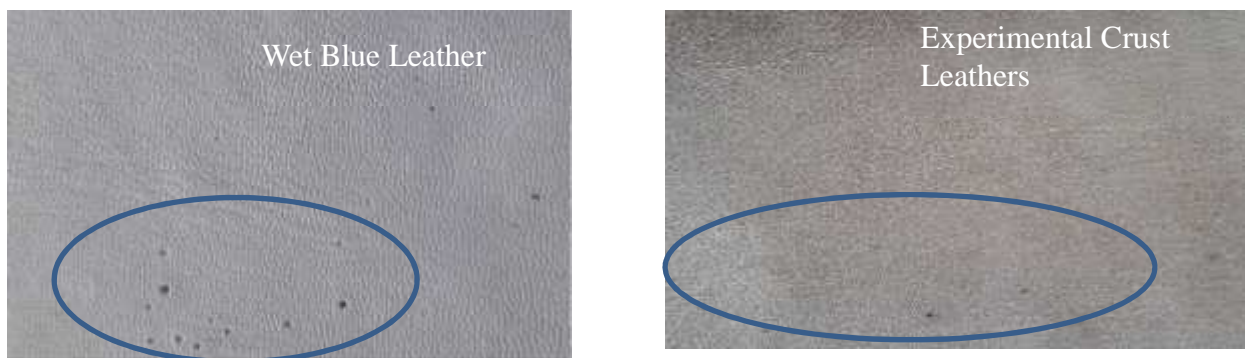
Figure 4.3 Wet blue leather with surface defects and dyed crust leather control
