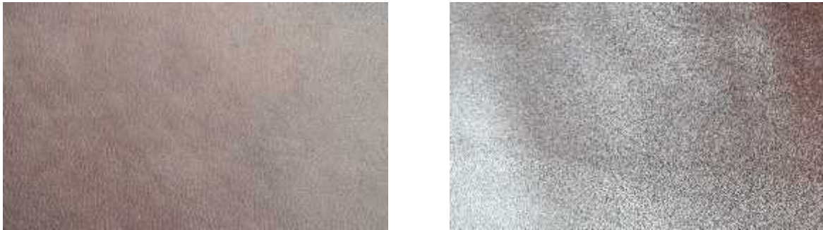
Fig 4.16 a) Dyed crust leather ready for metallic finishing and b) Metallic finished leather
