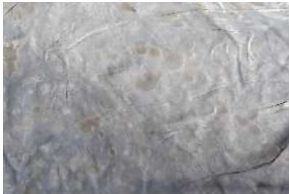
Figure 2.3 Semi-processed pickled sheep skin from M/s Colba Tannery, Modjo showing defects due to infectious pox diseases causing a flamed spot on the entire skin surface
