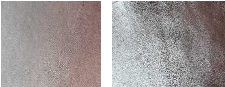
Fig 4.19 a) Dyed crust leather for resin finishing and b) Resin finished leather
