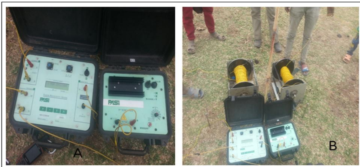
Figure 4.1 (a) PASI-16 GL and P-100 energizer instrument and (b) during field survey with cables and reels.
