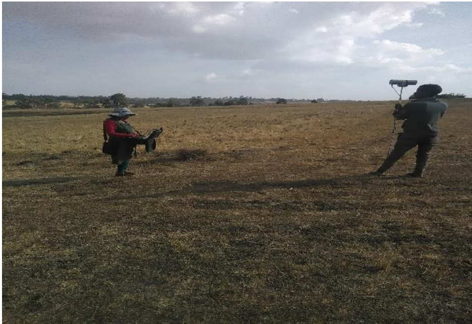
Figure 4.3 Magnetic data acquisitions at field using proton precession magnetometer-600
