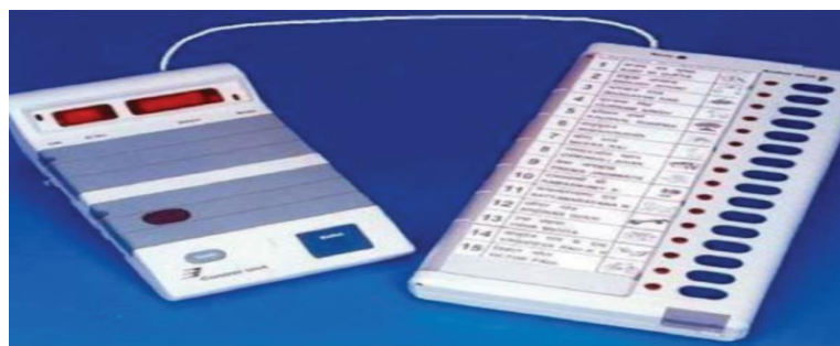
Figure 2- 3: Electronic Voting Machine used by Namibian 2014 general election (Ballot Unit on the left and Tabulator on the right)
