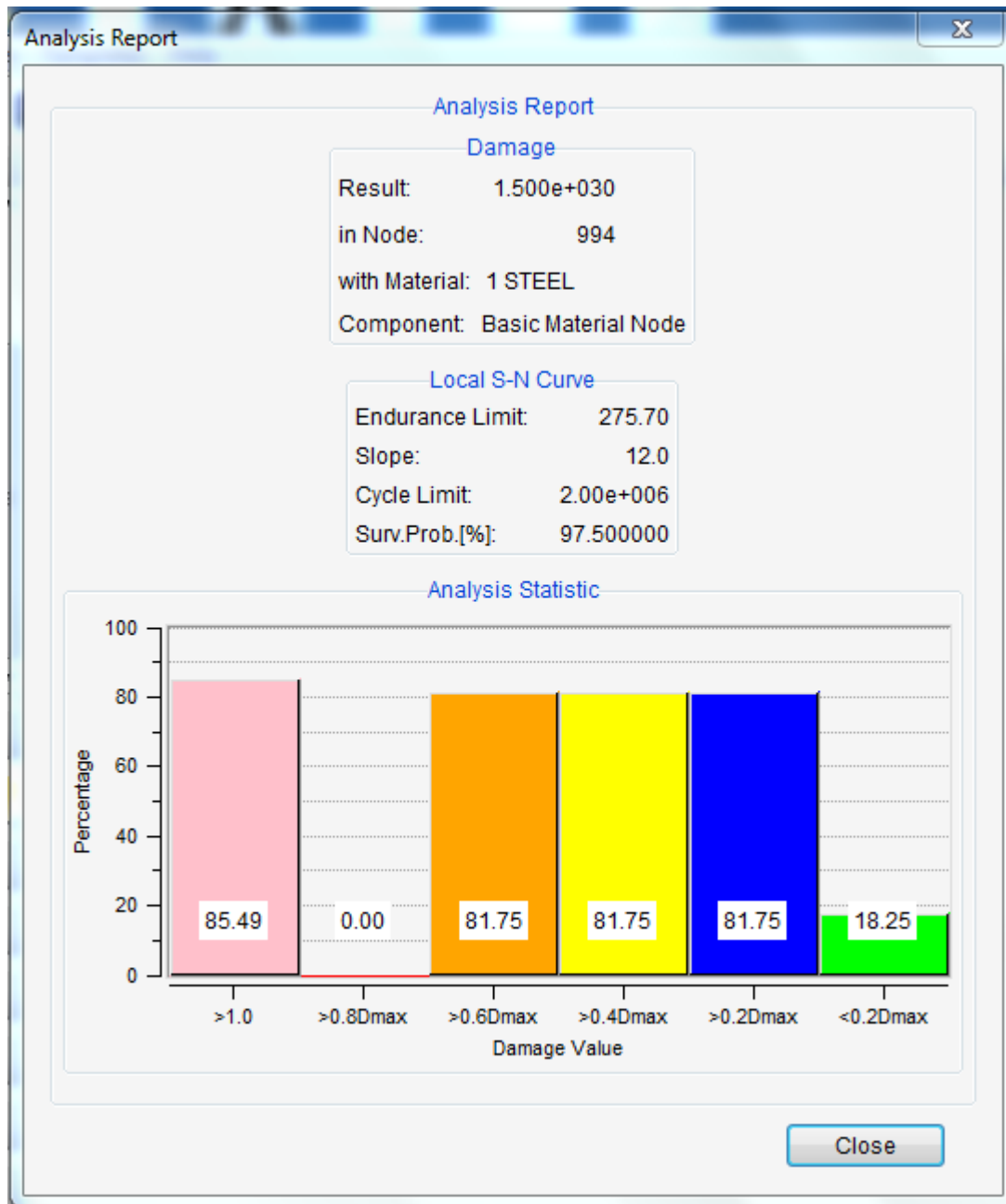
Fig. 4.37 damage analysis report at small seam thickness sensitivity
