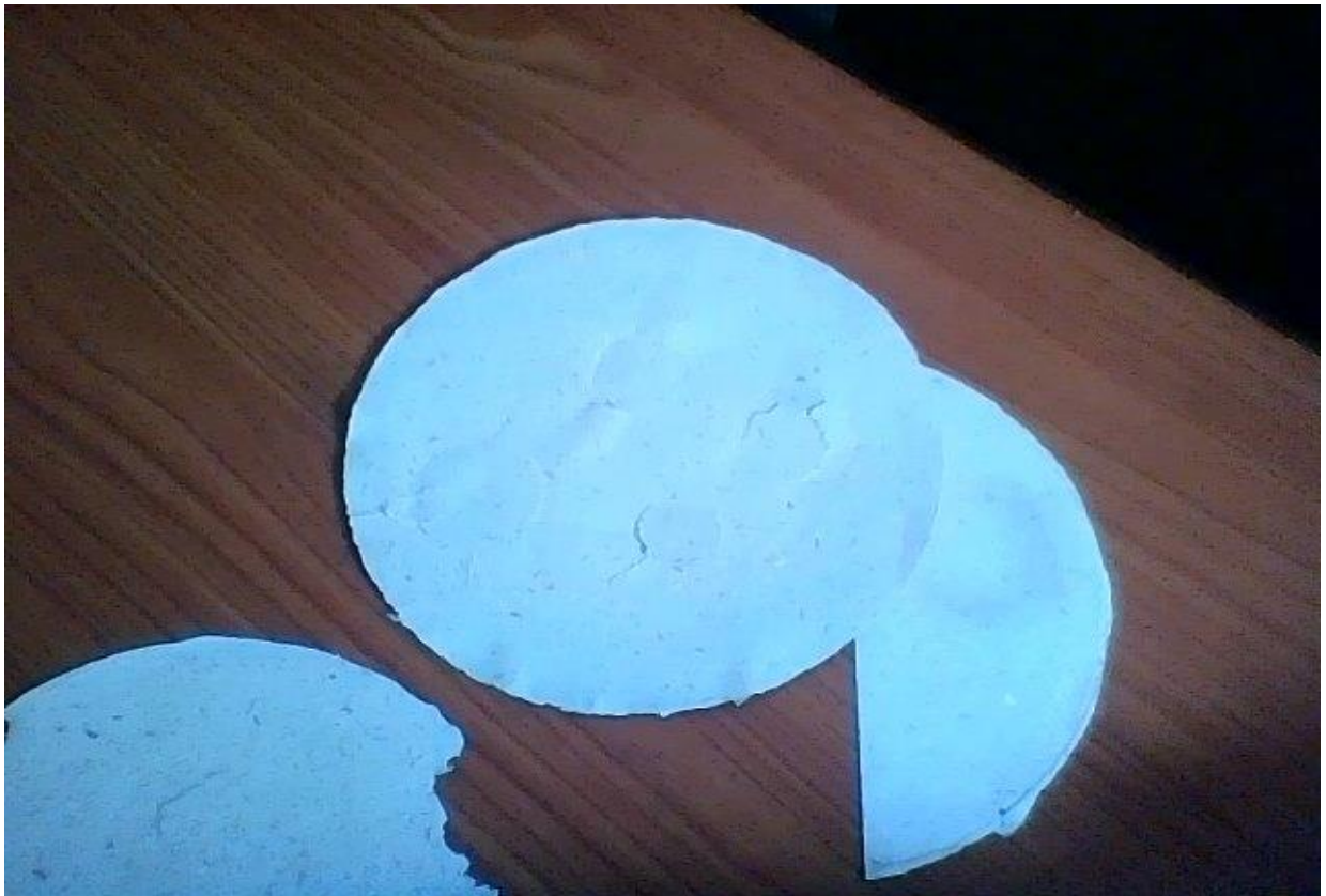
Figure 4.15: cotton stalk pulp hand sheets tested for physical strength indices
