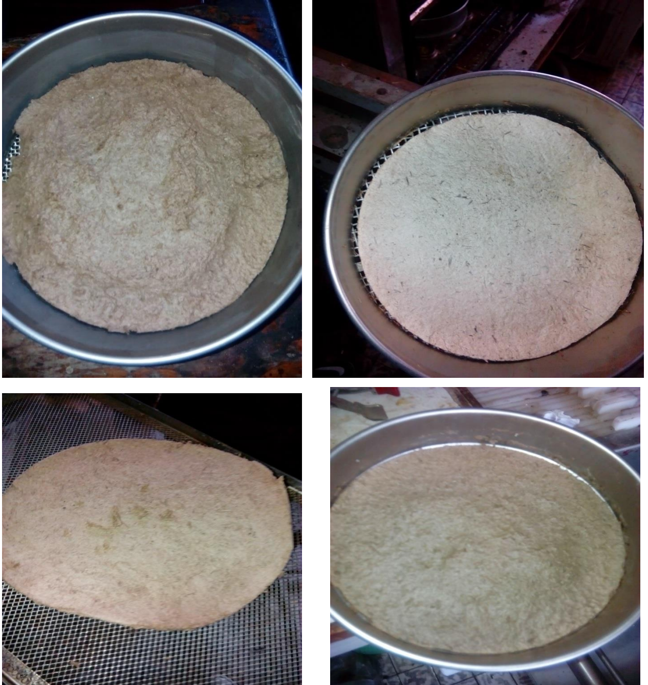
Figure 4.2: Cotton stalk pulps dried by oven
