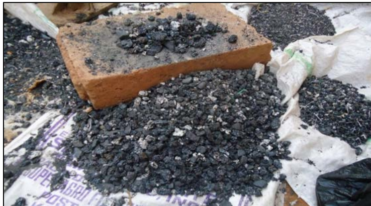
Figure 3-2: Waste steel slag aggregates crushed to different sizes
