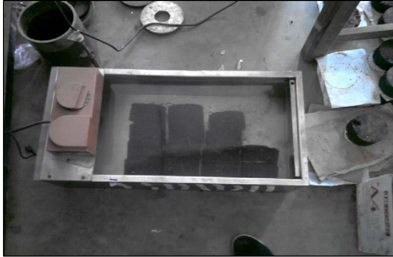
Figure 3-5: Water bath conditioning for 24hours
