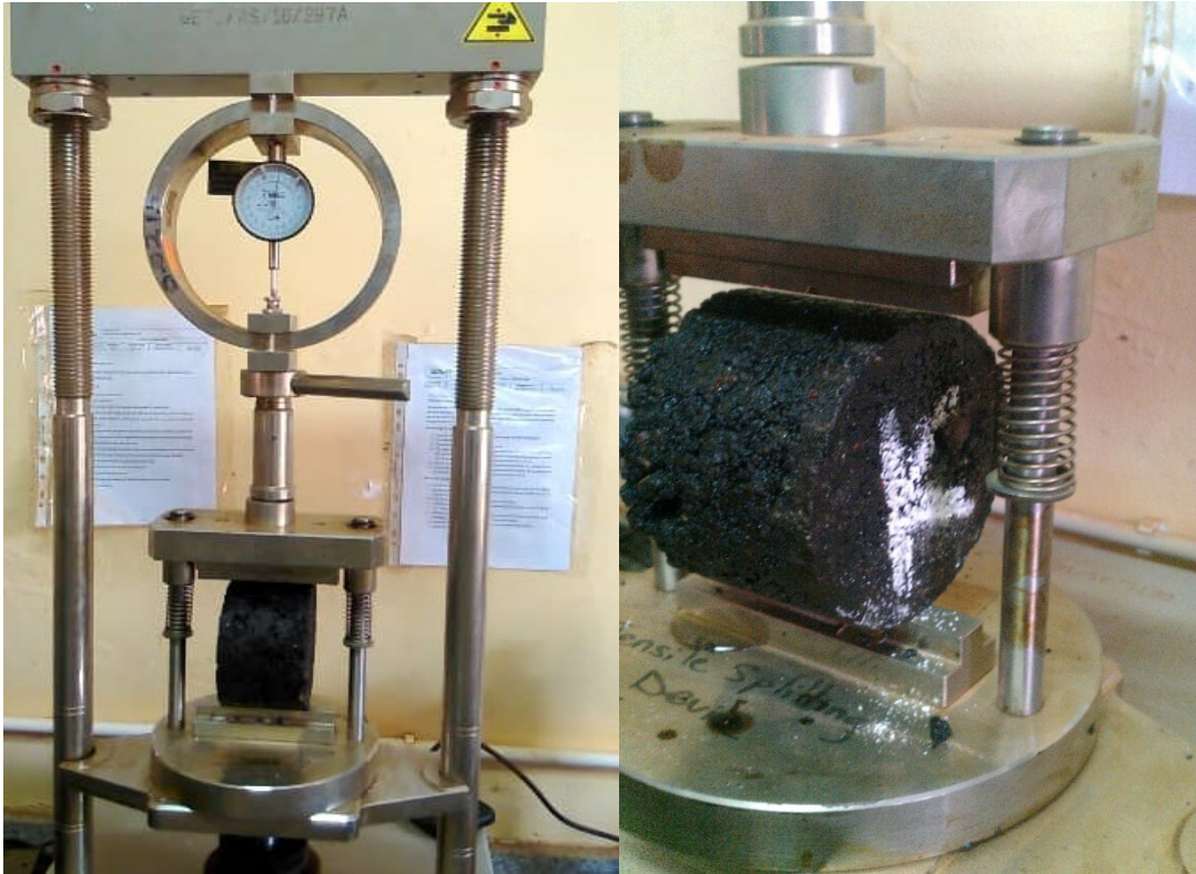
Figure 3-4: Diametric loading of Marshall Specimen under Indirect Tensile Strength test
