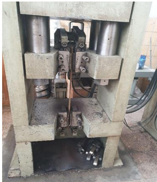
Figure 3-3: Testing tensile strength of bar used.
