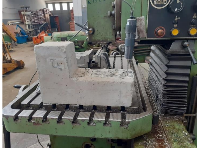
Figure 3-24: Measuring depth using displacement transducer.
