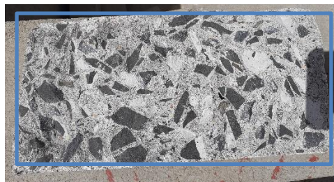
Figure 4-20: Failed surface for cast with interface sample and tensile area of 150 mm length and 100mm width.
