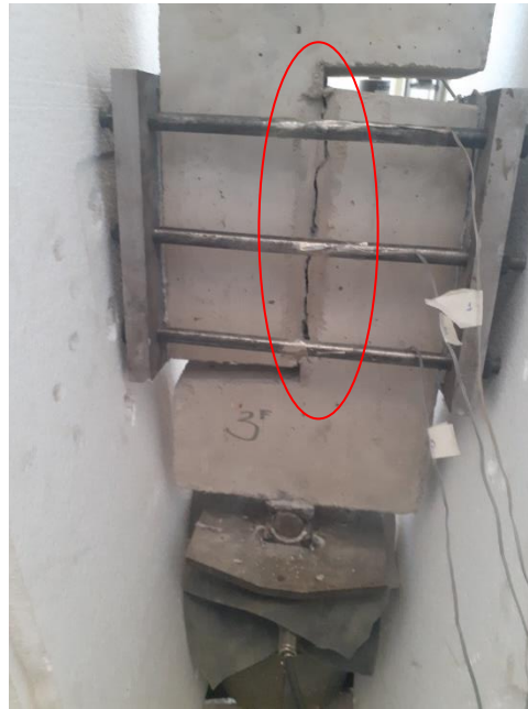
Figure 4-14: Crack pattern of the shear test.
