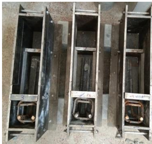
Figure 3-9:Placing of reinforcement.
