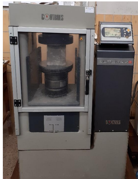
Figure 3-15: Strength test machines a) cylindrical splitting tensile(left) and b) cubic compressive strength(right).
