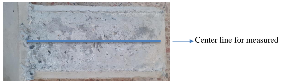
Figure 4-22: Shear area for monolithically cast cracked sample.
