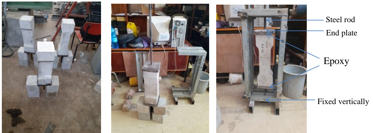
Figure 3-21: Attaching plates to the sample with epoxy (a) bottom epoxy (b) top epoxy (c) testing frame.
