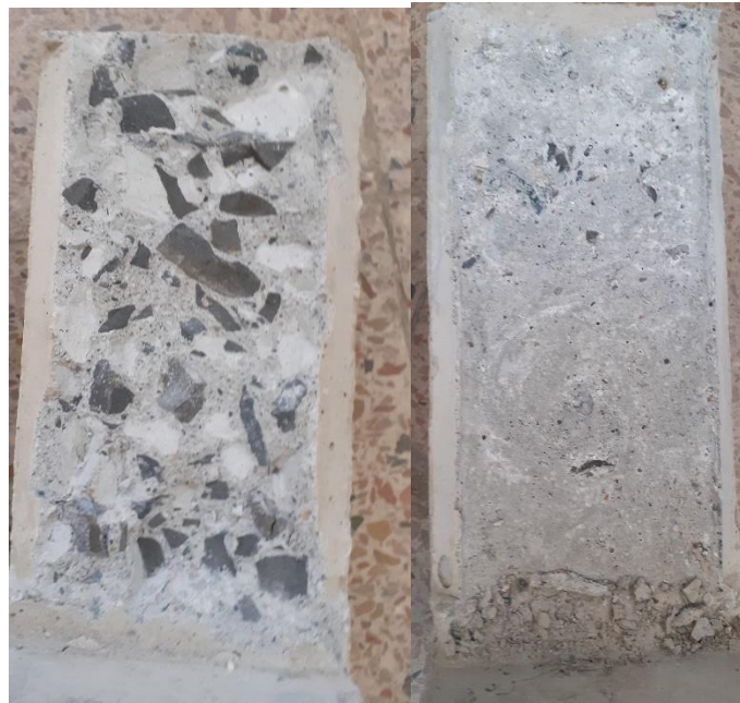
Figure 4-14: Crack pattern of the shear test.
