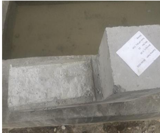
Figure 3-10:Substrata structure after remove from the mold.
