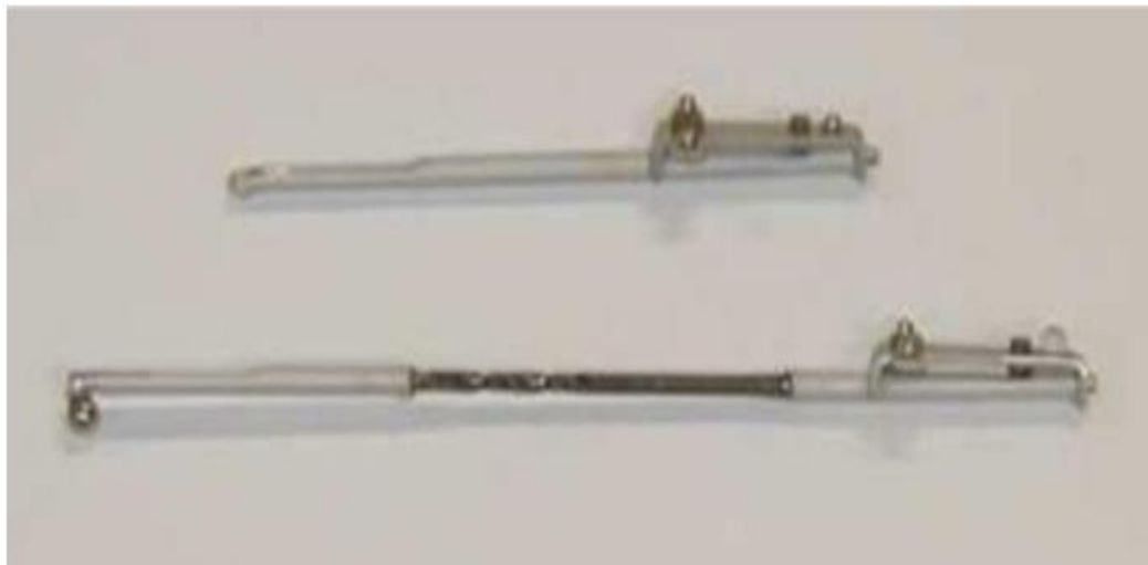
Figure 2-16: Two types of profilometer styluses(Courard, Bissonnette, & Garbacz, 2015).
