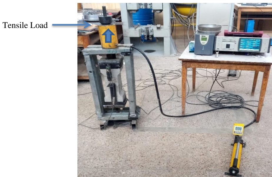
Figure 3-22: Direct tensile setup using center hole jack.
