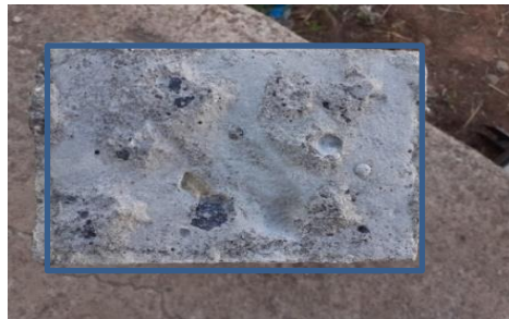
Figure 4-19: Crack pattern of failed samples.
