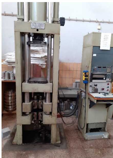
Figure 3-15: Strength test machines a) cylindrical splitting tensile(left) and b) cubic compressive strength(right).
