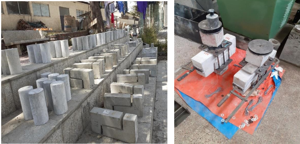
Figure 3-18: specimen after curing and epoxy.
