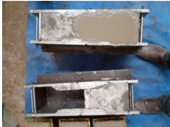
Figure 3-14: Casting of new concrete
