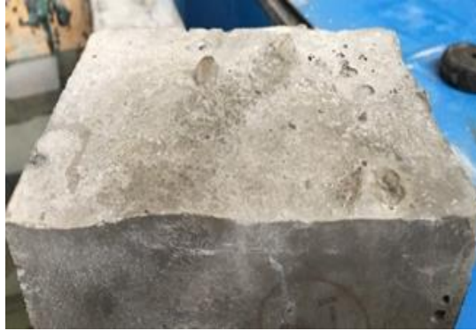
Figure 3-13: Surface roughness at tension zone.
