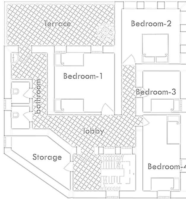
Figure 42: Hypothetical first-floor plan prepared as per the findings (Source: Fieldwork Measurement & Drawing by The Data Collectors)
