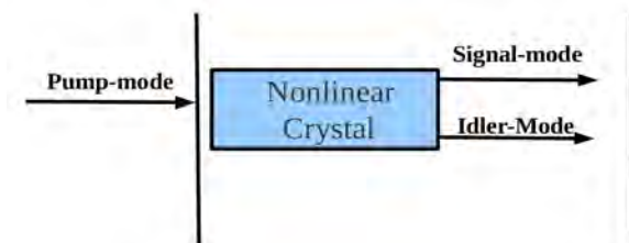
Figure 3.1: Two-mode subharmonic generator
