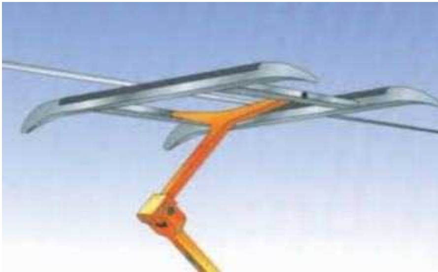
Figure 2.1: Sliding contact of the contact strip against contact wire [10].
