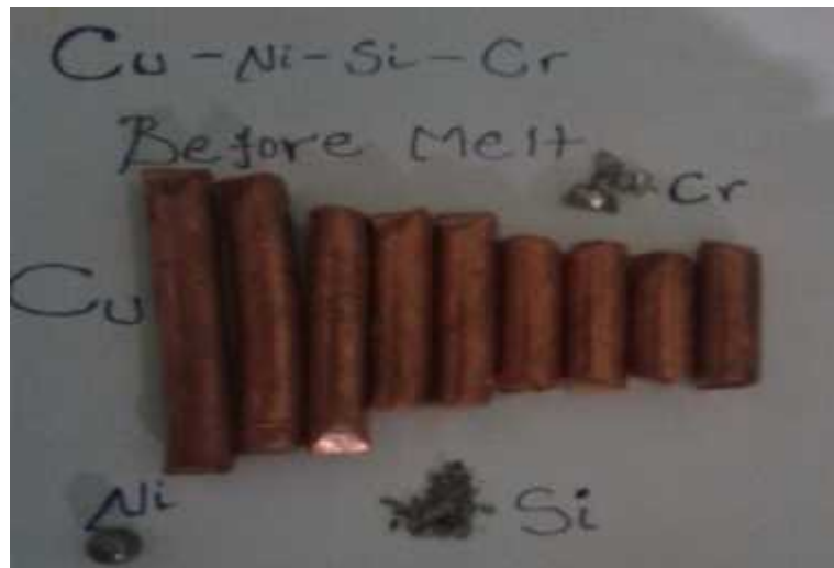
Figure 3.2: Composition of pin material Cu-Ni- Si-Cr before melting process.
