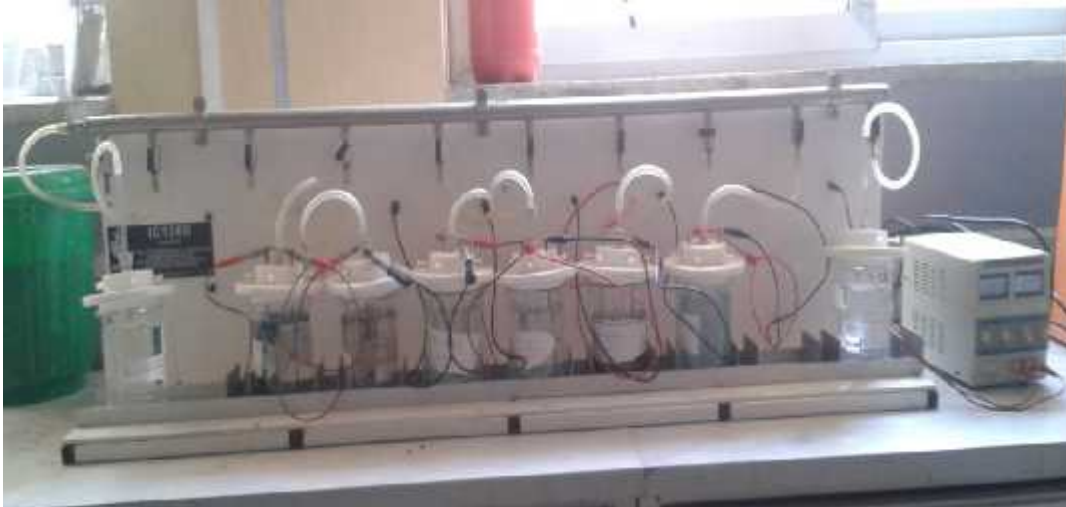
Figure 3.10: Test pieces in different test solution media.
