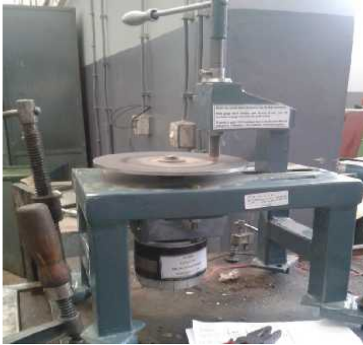
Figure 3.11: Pin on disc tribometer when the pin slides on the disc.
