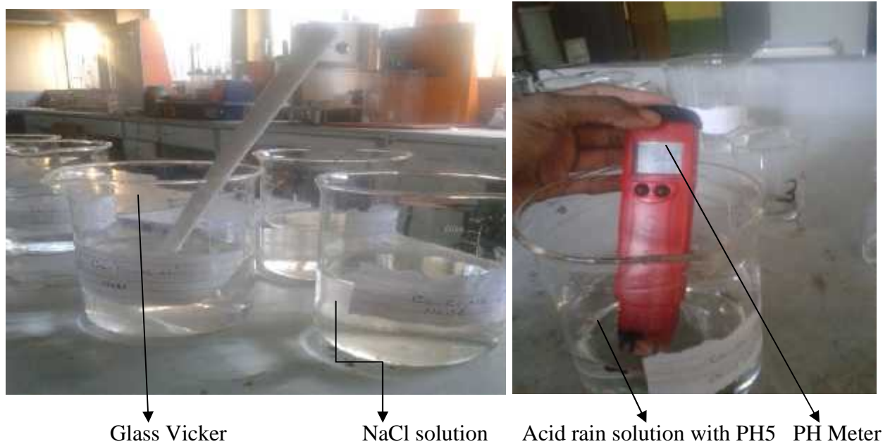
Figure 3.9: Preparation of test solution media PH value and acid adding process.
