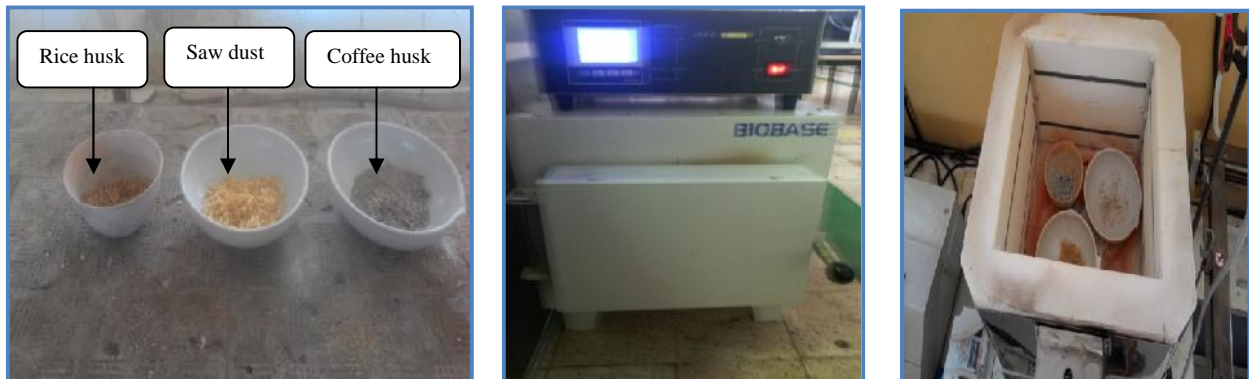
Figure 3-3: Volatile mater content determination experiment
