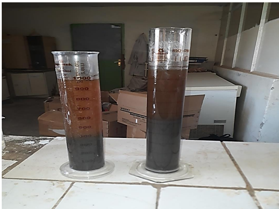
6. 7: Photo of the clarified filtrate juice at 6 ppm of flocculant and LFJ of 7. 10 pH
