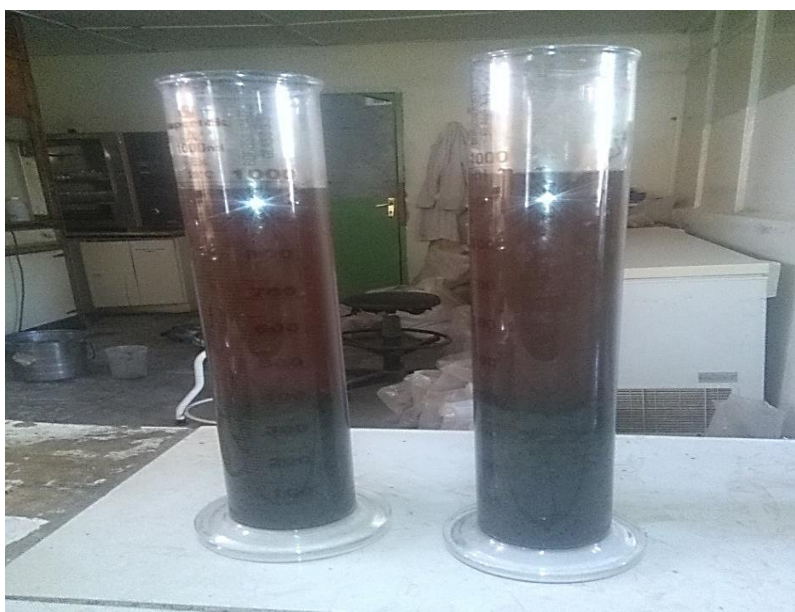
6. 8: Photo of the clarified filtrate juice at 6 ppm of flocculant and LFJ of 6. 68 pH
