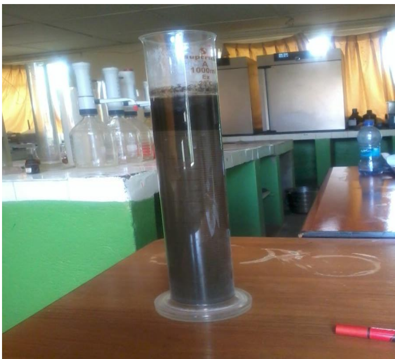
6. 9: Photo of the clarified filtrate juice at 3.17ppm of flocculant and LFJ of 7.10 pH
