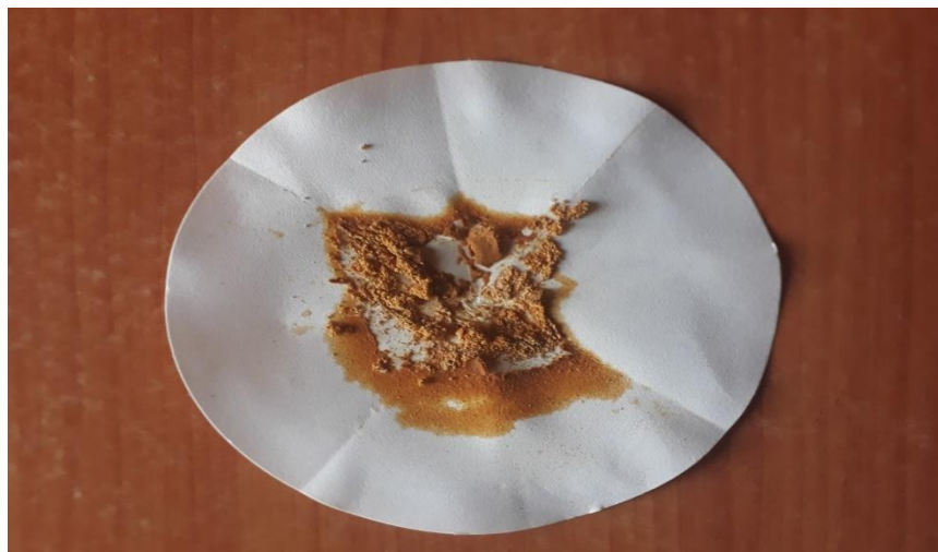
6. 10: Photo of insoluble solid filtered from 10grams of lime
