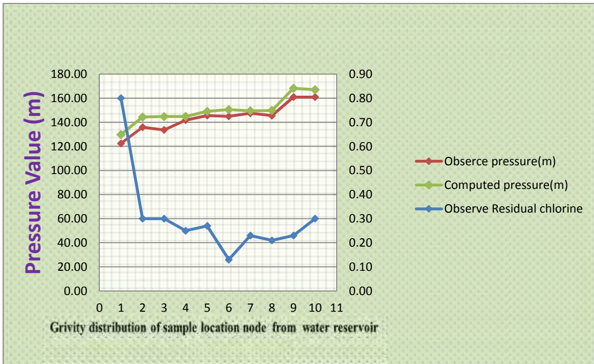
Figure 4-23: Relationship between pressure changes with residual chlorine in the distribution network system
