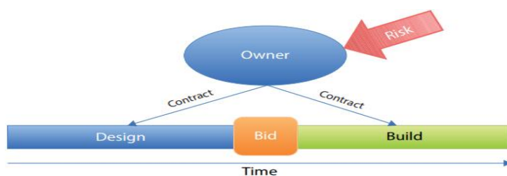
Figure 2.1: Design-Bid-Build Project Delivery Method
