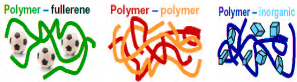
Figure 3.4: Schematic view of types of CP solar cells.
