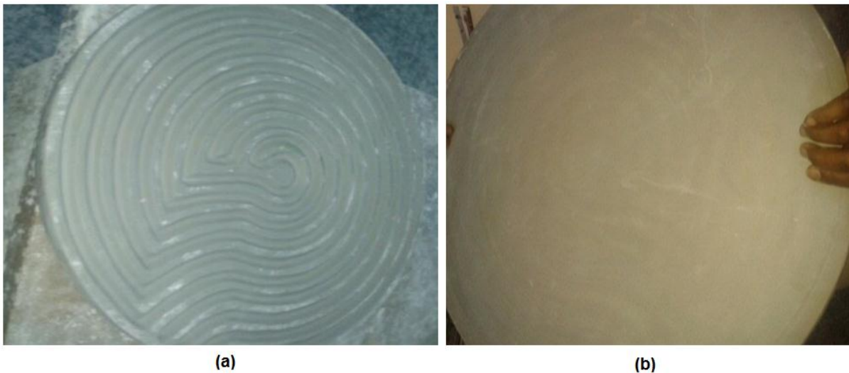
Figure 5-1: The bake ware (Mitad). Bottom of the bake ware with the built in grove (a) and top surface of the bake ware before smoothing (b)
