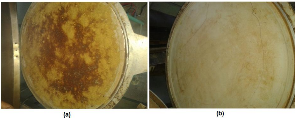
Figure 5-3: Pretreatment of the bake ware before baking. Burning of gomenzer (powdered oil seed) on the surface of the bake ware (a) and the final smoothed and hardened surface (b)
