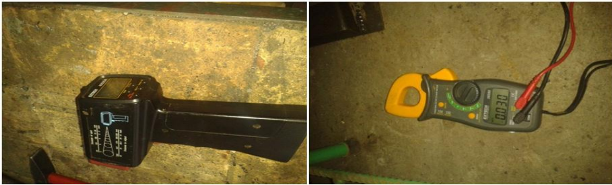
Figure 5-6: Temperature measurement instruments. Infrared thermometer (Left) and Multi -meter (Right).
