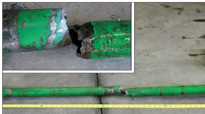
Figure 2.2: Critical speed failure of a driveshaft that resulted in buckling failure [34]
