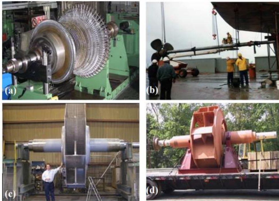
Figure 1.1: Typical applications of rotors: (a) turbo-machinery (different stages); (b) ship propeller shaft; (c) backward curved fan; (d) gas recirculation fan [6]
