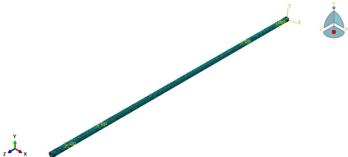
Figure 3.5: meshed shaft for Torsion and bending
