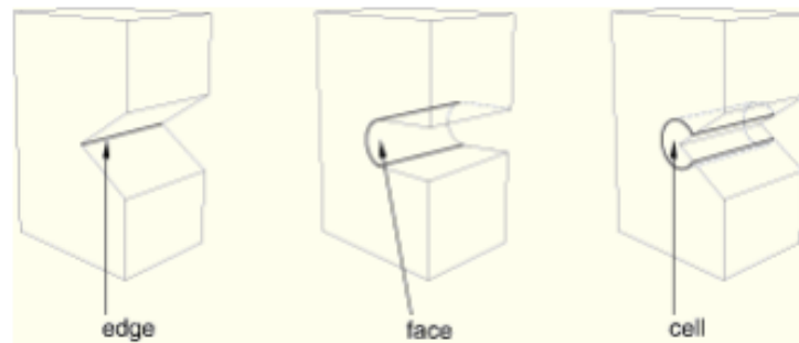
Figure 2.10: crack selection for contour integral
