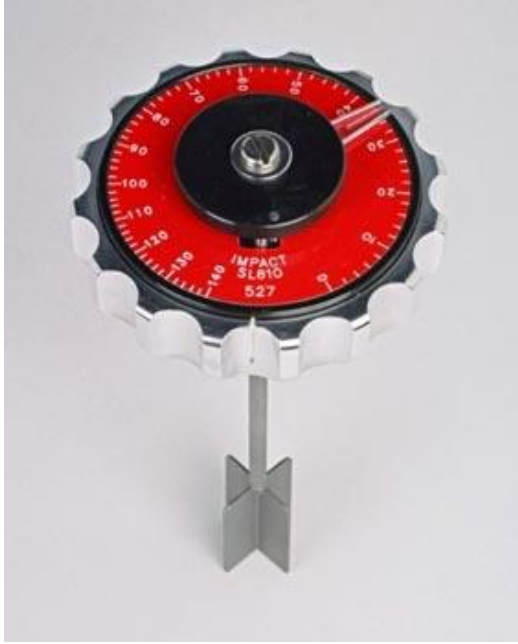
Fig 2.3 Field vane shear test equipment
