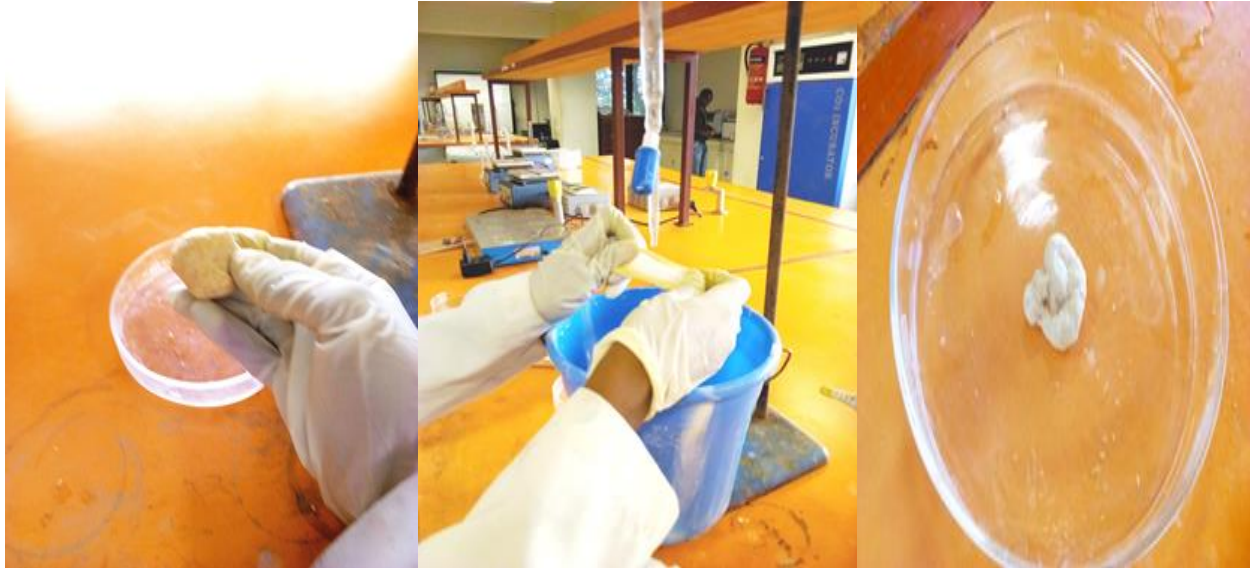
Figure: 3.2. Determinations of wet gluten from ball of dough of Triticum aestivum L. flour by hand wash method
