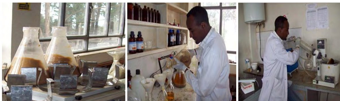
Figure 3.2: Photograph showing different steps of extraction through orbital shaker, filtration and crude extraction by Rota vapor.
