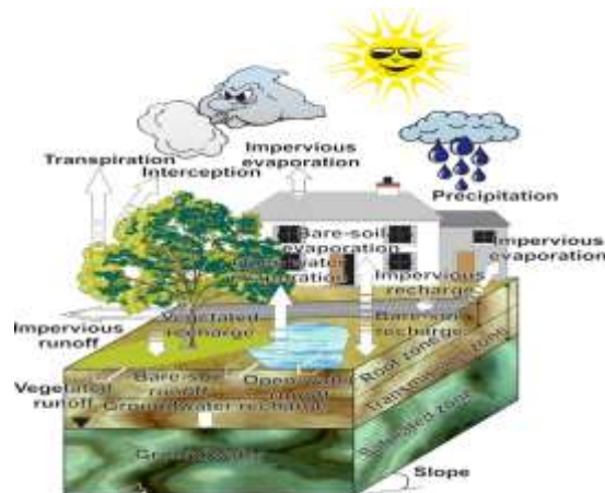
Figure 1. Schematic WB of an hypothetical raster cell (after O.Betelaan and D.Smelt 2007)
