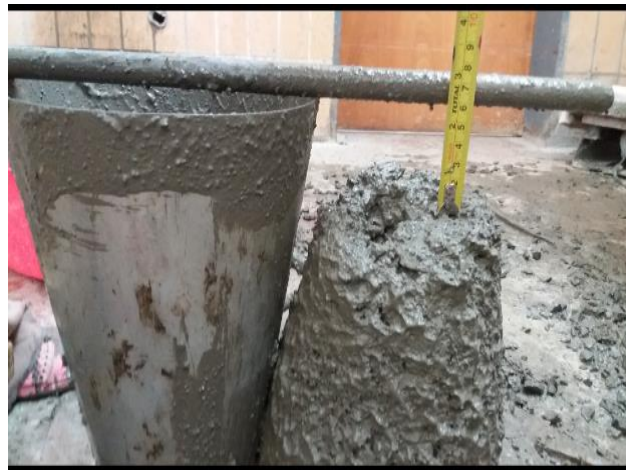
Figure 3-9 Slump test on mixed fresh concrete
