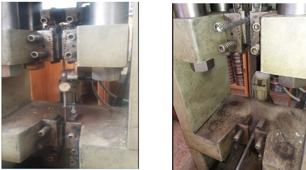
Figure 3-8 Universal testing machine test set up at AAIT
