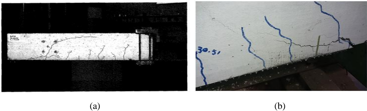
Figure 6-2 (a) failure of specimens tested by Jansze (b) failure of GK-RET5 series specimens
