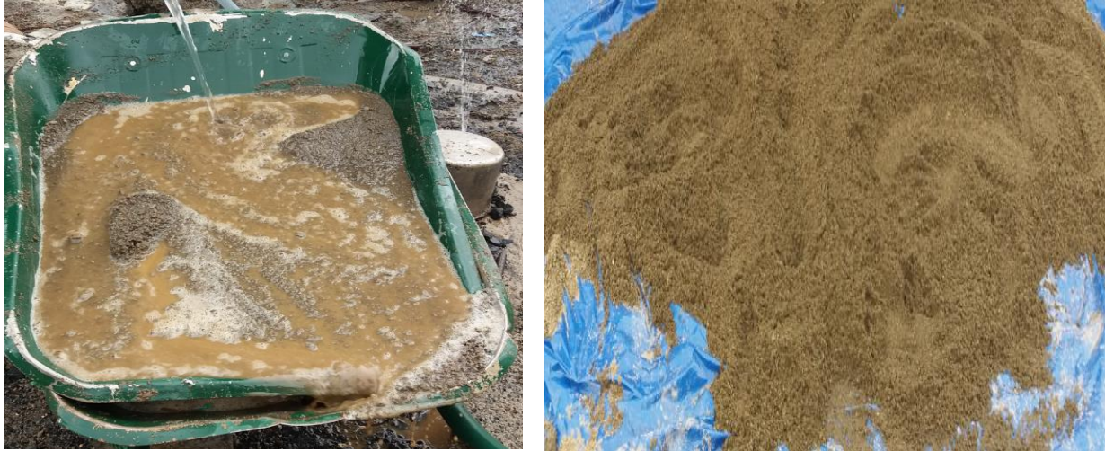
Figure 3-6 washing treatment of fine aggregates
