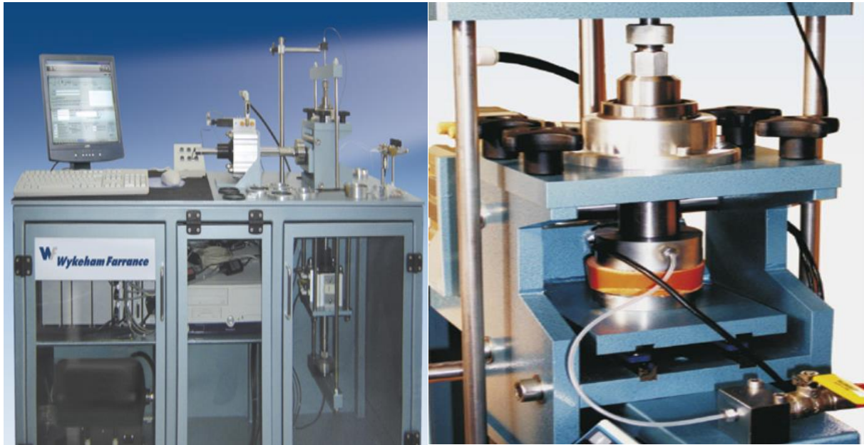
Figure-3-1: 31-WF7500 cyclic simple shear machine. (Seinwill, 1984)
