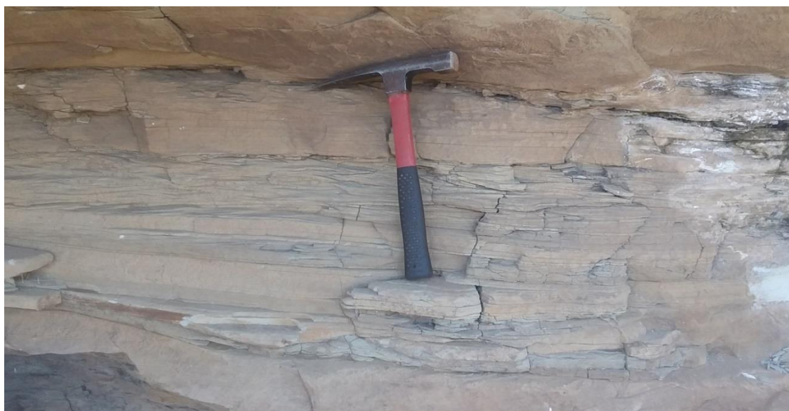
Figure 5.5 field photograph of thinly bedded sandstone from the bottom of the section
