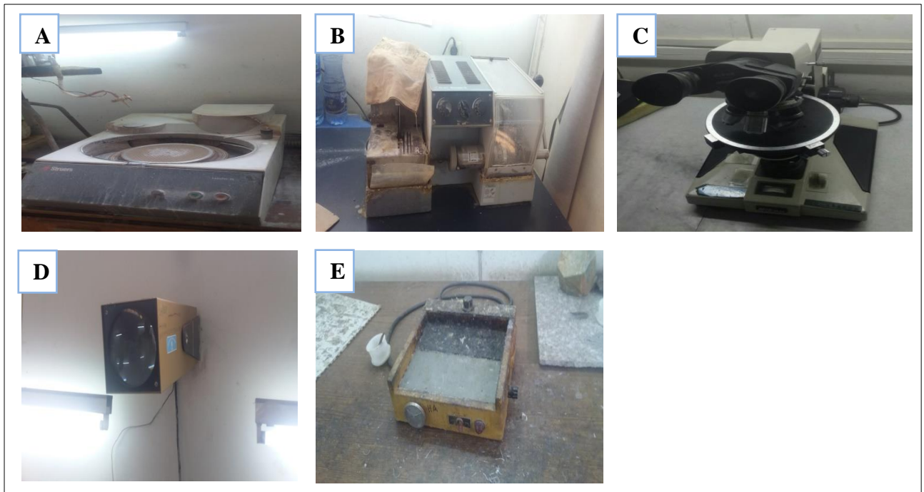
Figure 1. 6 Laboratory Equipment's used in the preparation of the thin section of the rock, A, grinding machine B, Cutting slab C, petrographic Microscope D, petrographic light source E, hot plate
