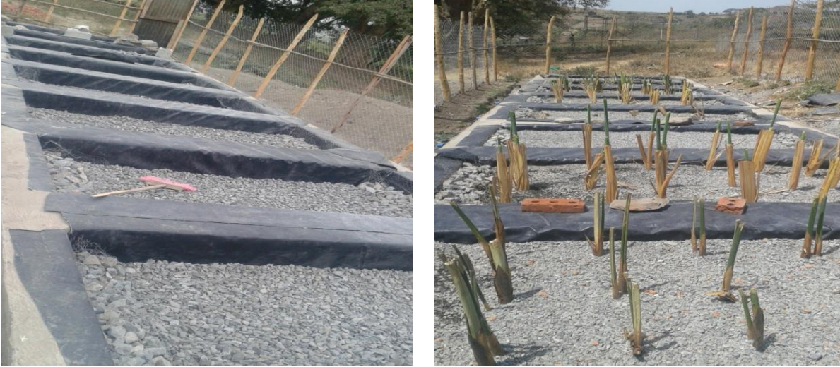
Figure 7. Photographic presentation of the Pilot scale subsurface flow constructed wetlands
