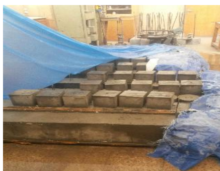
e) Concrete in curing
