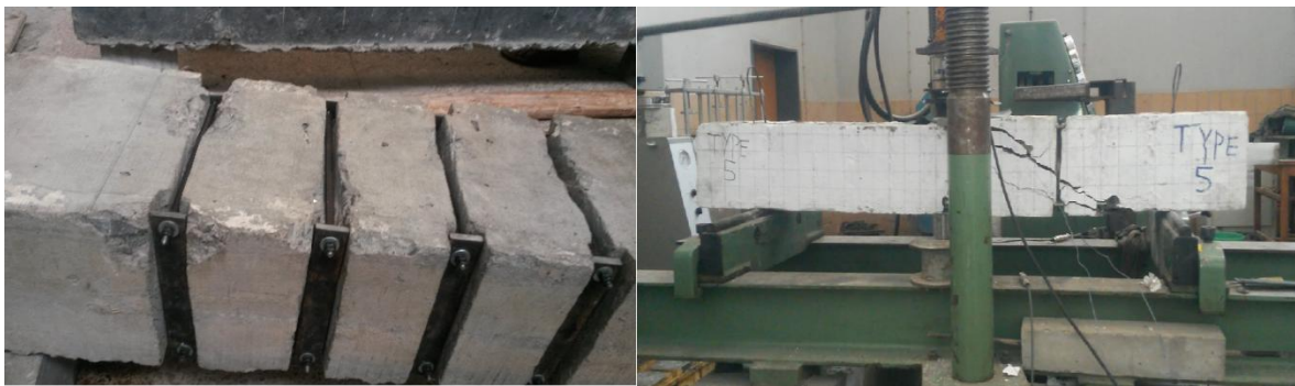
Figure 5.5: Staggered Vertical Stirrups only Provide along Shear Span by Drilling (Beam Type-5)
