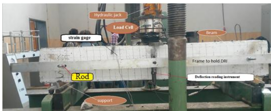
Figure 3.13: Loading Setup
