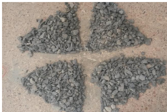
b) Quartering of aggregate
