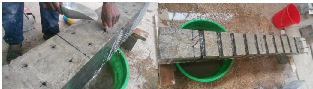
Figure 3.9: Drilled and Grooved Wash from Dust
