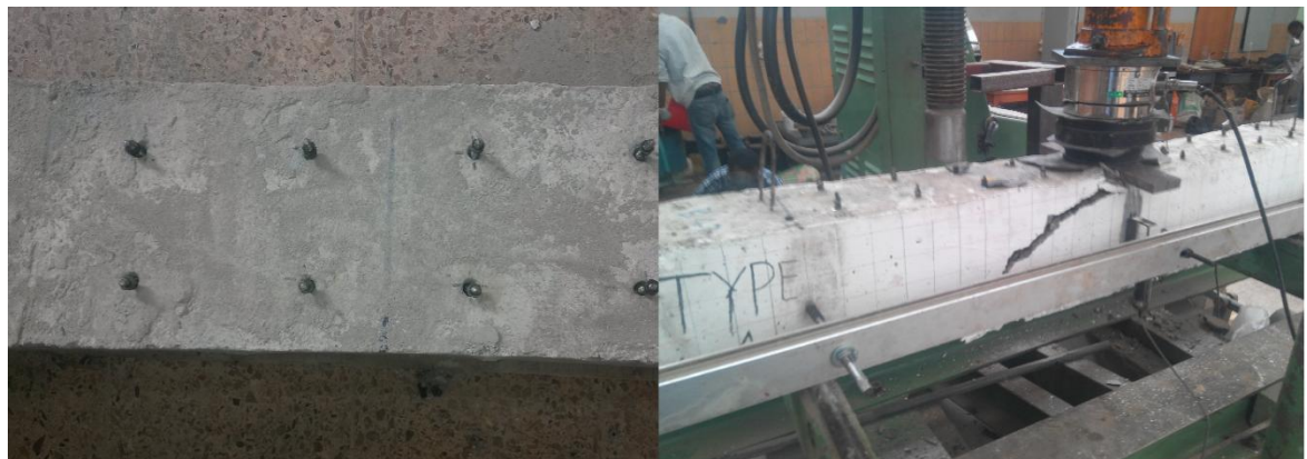
Figure 5.3: Parallel Vertical Stirrups and Horizontal Plate Provide along Shear Span by Drilling (Beam Type-3)
