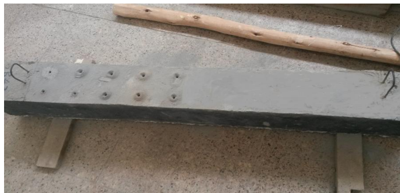
Figure 5.10: One Side of Shear Span Drilled and the Other Side Undrilled Beam
