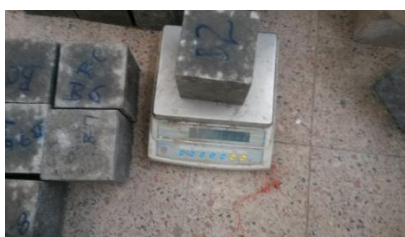
Figure 3.7: Cubes Weighted for Test Compressive Strength
