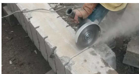
b) Specimen grooving
