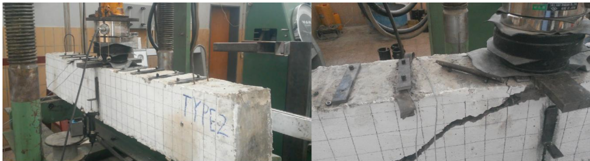
Figure 5.3: Parallel Vertical Stirrups and Horizontal Plate Provide along Shear Span by Drilling (Beam Type-3)
