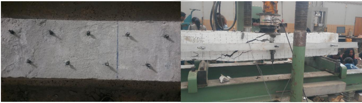
Figure 5.5: Staggered Vertical Stirrups only Provide along Shear Span by Drilling (Beam Type-5)
