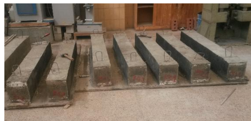
d) Removed formwork
