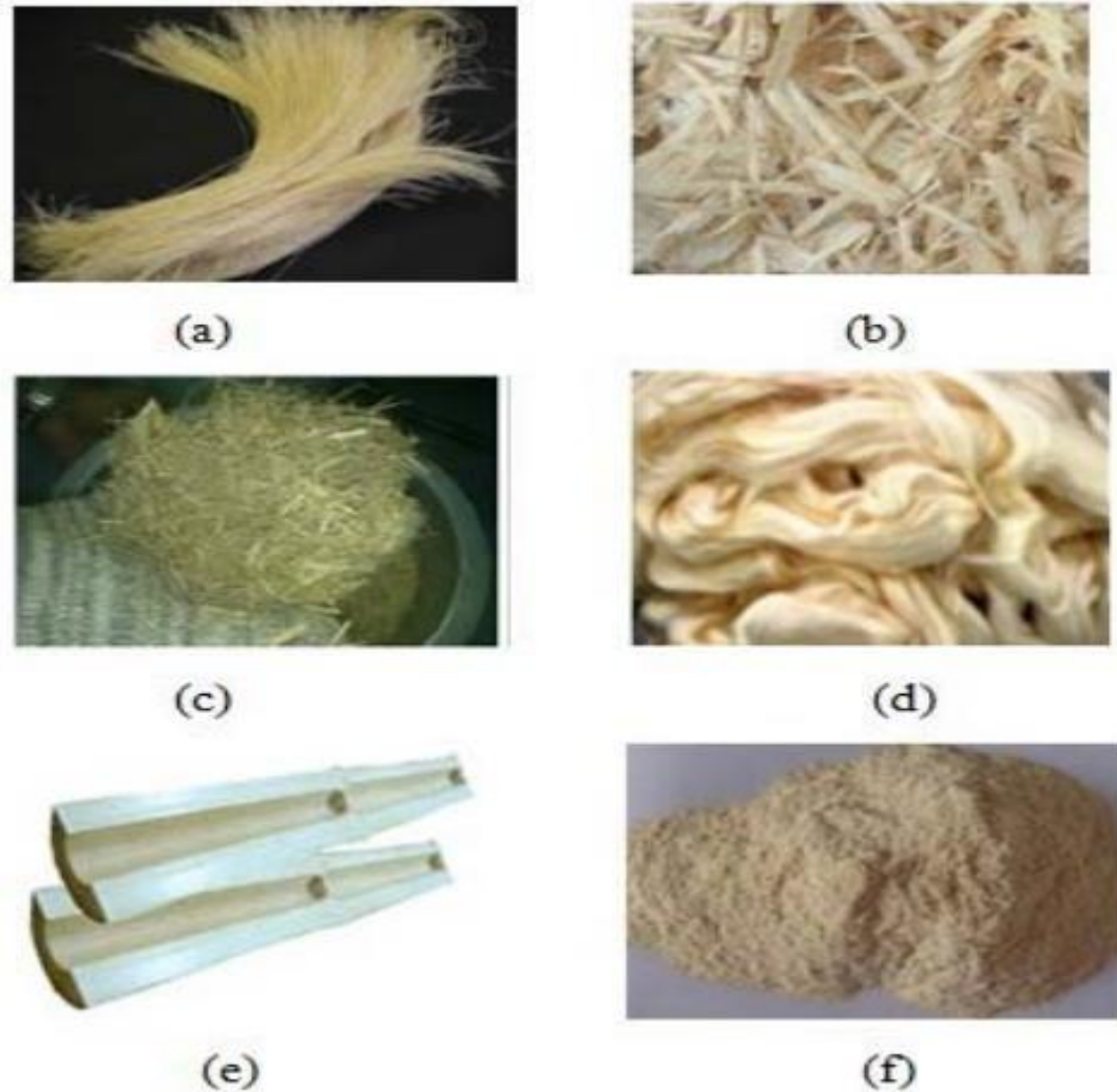
Fig.3.1: Forms of bamboo being used as composite reinforcement (a) long fibers (b) flake (c) short fibers (d) sliver (e) strips and (f) powder. [21]
