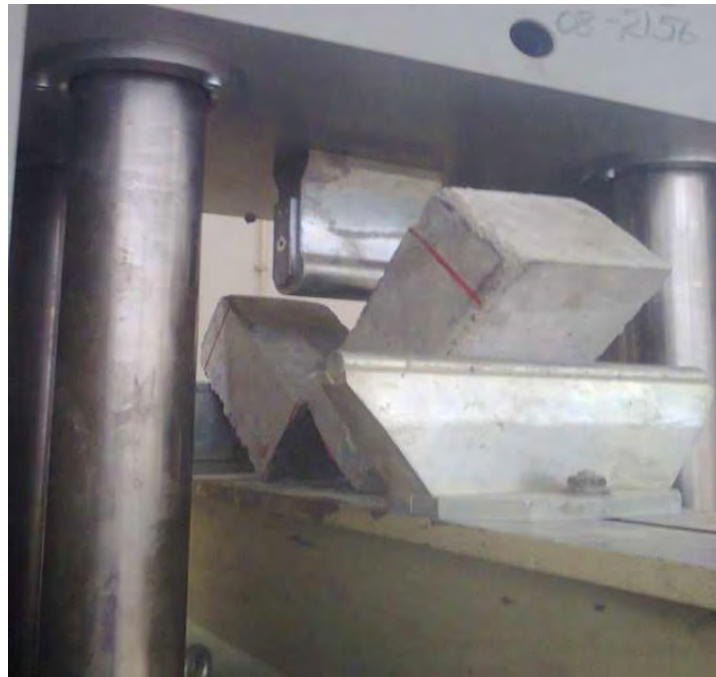
Figure 4.10: Center point loading flexural strength test
