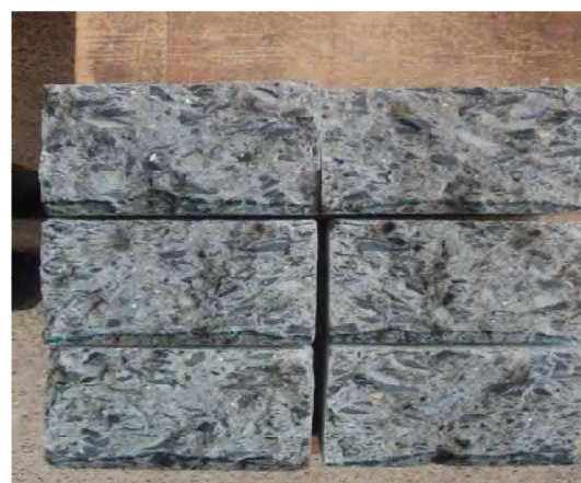
Photo: Water penetrated sample
