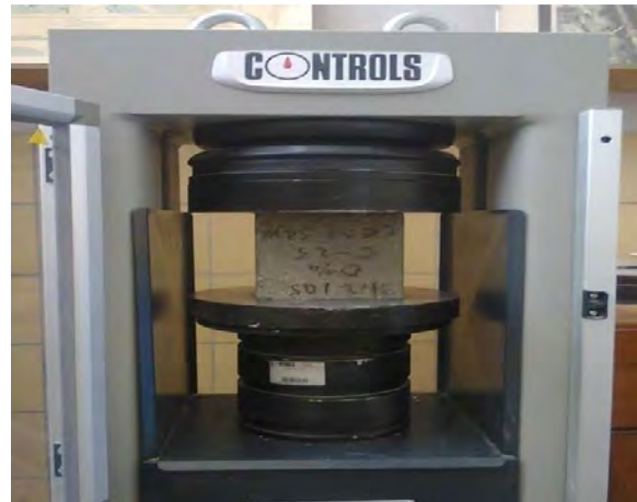
Photo: Concrete ready for compressive strength test
