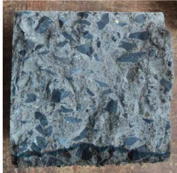
Figure 4.14: Water penetrated sample
