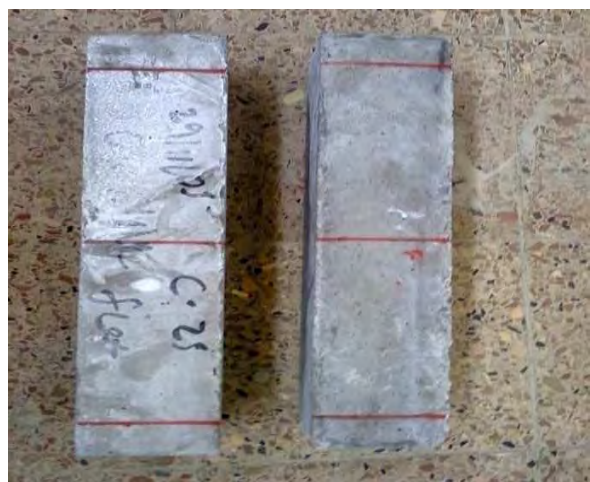
Photo: Flexural test concrete sample
