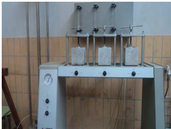
Photo: Sample ready for permeability tests
