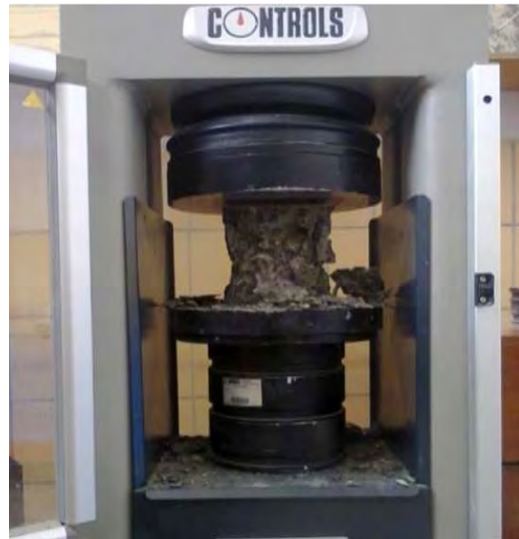
Figure 4.2: concrete cube sample after testing
