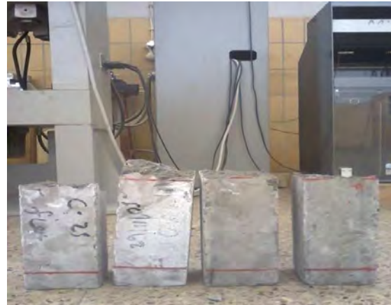
Photo: Sample after flexural strength test
