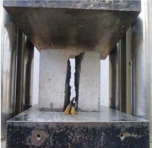
Figure 4.13: Sample after splitting
