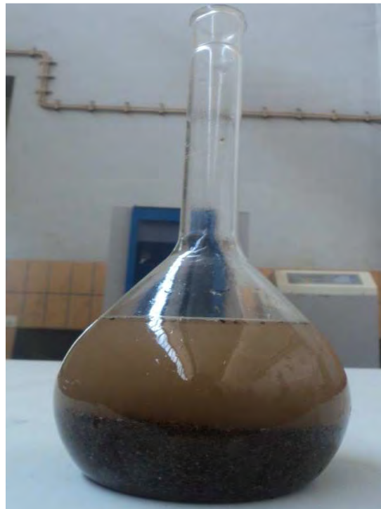
photo: Specific gravity test for fine aggregate
