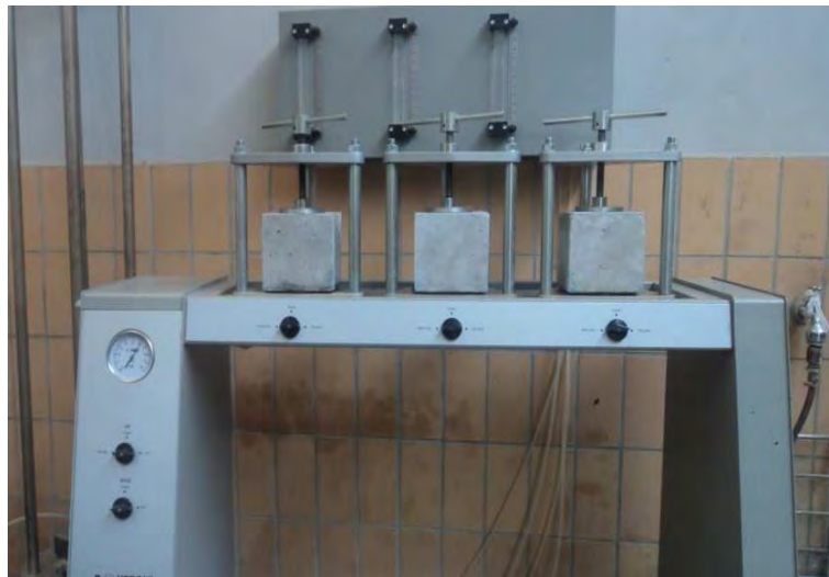
Figure 4.12: Typical concrete samples ready for permeability test.
