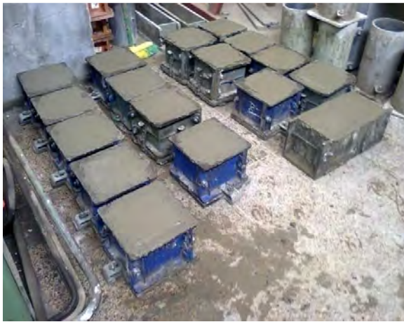
Photo: Casted concrete sample
