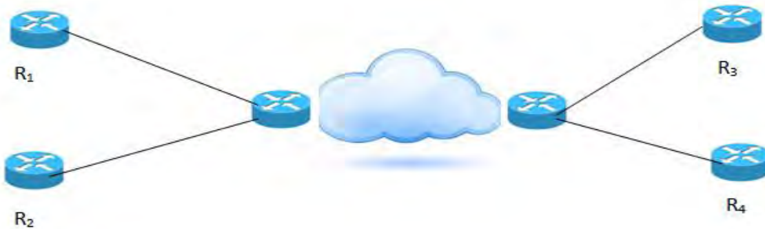
Figure 5.5: Routers' connection to show how jitter is measured in a network [22]
