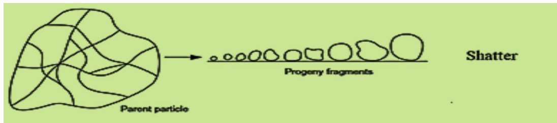
Figure 2: Fracture mechanism of the particles; shatter (Ghanei, 2019)
