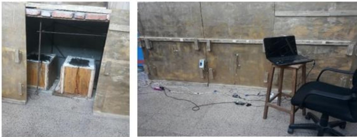
Figure 3.13 Final Setup of Temperature Chamber with its Full Controlling System
