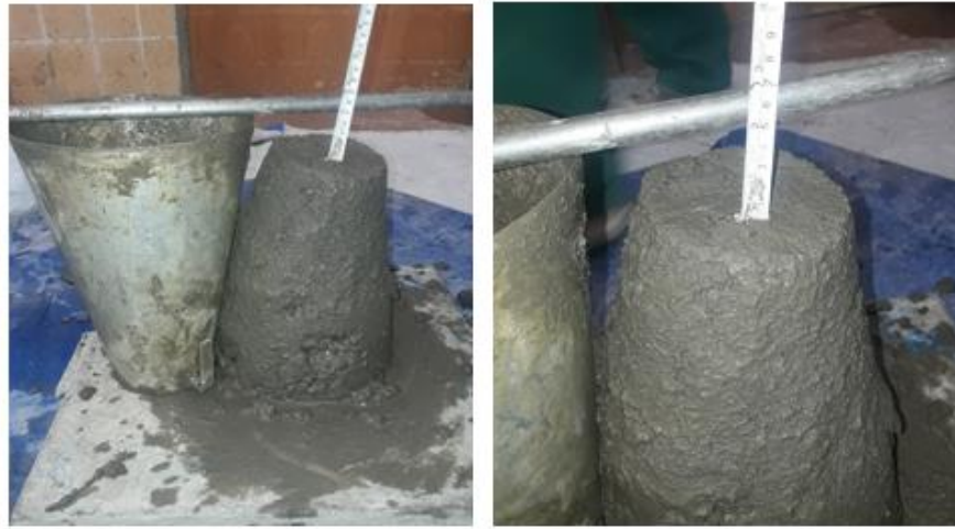
Figure 3.6 Measuring Slump of Fresh Concrete
