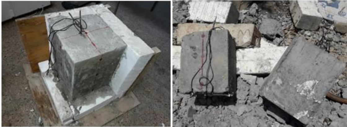
Figure 3.11 Demolding and Demolishing Concrete Samples for Reusing Thermocouples
