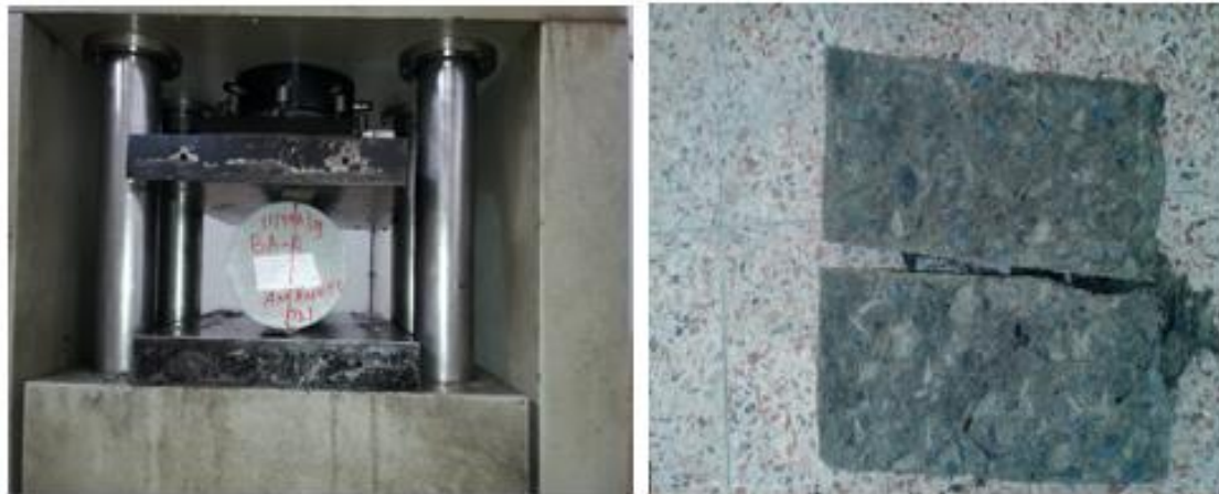
Figure 4.2 (a) Test Set up of Splitting Tensile Strength Test (b) Test Specimen after Failure
