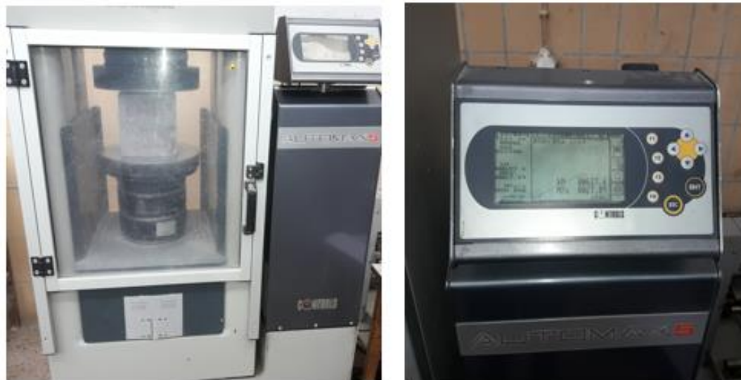
Figure 3.8 Compressive Strength Test Setup
