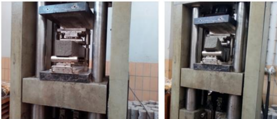
Figure 3.9 Flexural Strength Test Setup
