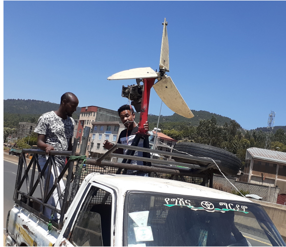
Figure 5.9: Set up of the turbine for experimental testing on the moving vehicle
