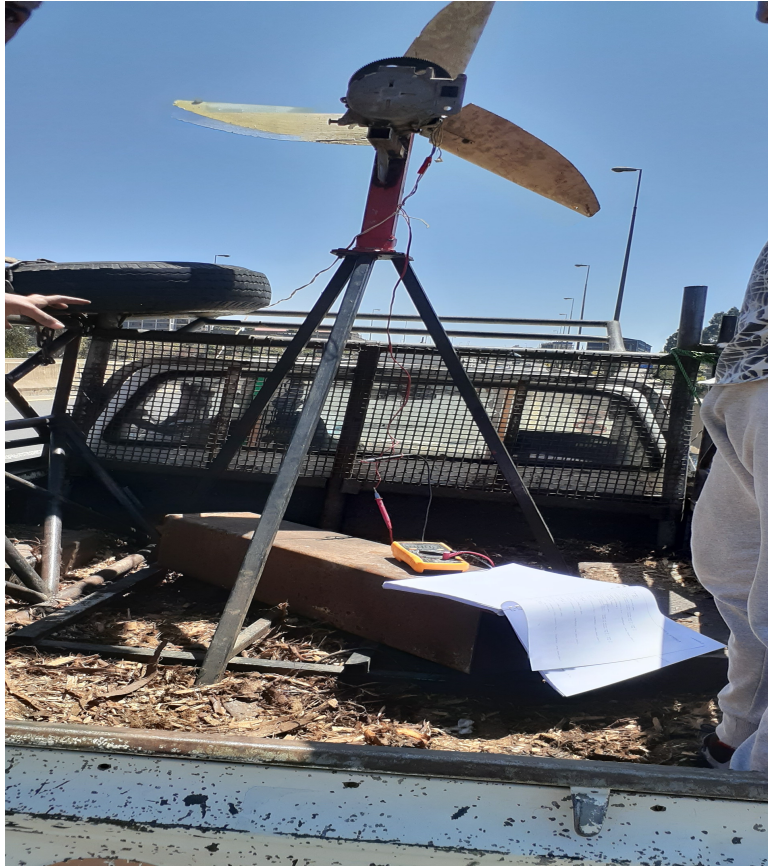
Figure 5.10: Measuring the voltage drop from the generator with multi-meter
