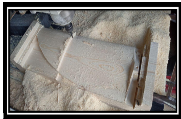
Figure 5.6: manufacturing of the designed blade with CNC machine
