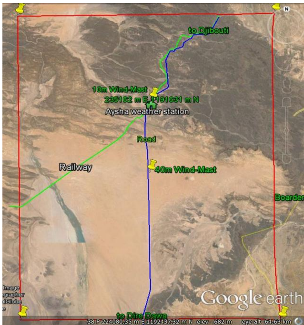
Figure 1.2: Area considered for the construction of wind farm with gravel road access map of the site [Google Earth]
