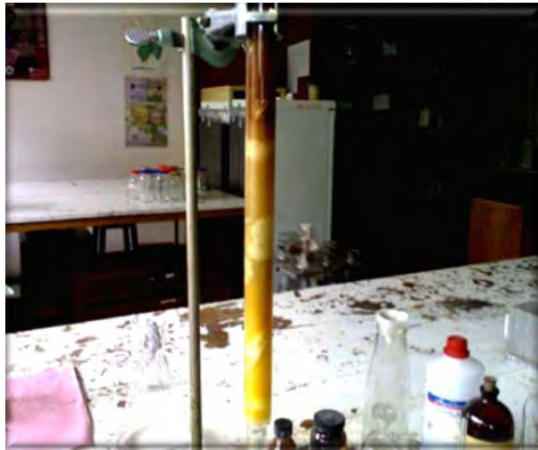
Figure 12. Isolation of bioactive compound (yellow) using CC
