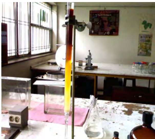
Figure 3. Purification of the bioactive compound using solvent system Petroleum ether: Chloroform (1:1 v/v) in column chromatography
