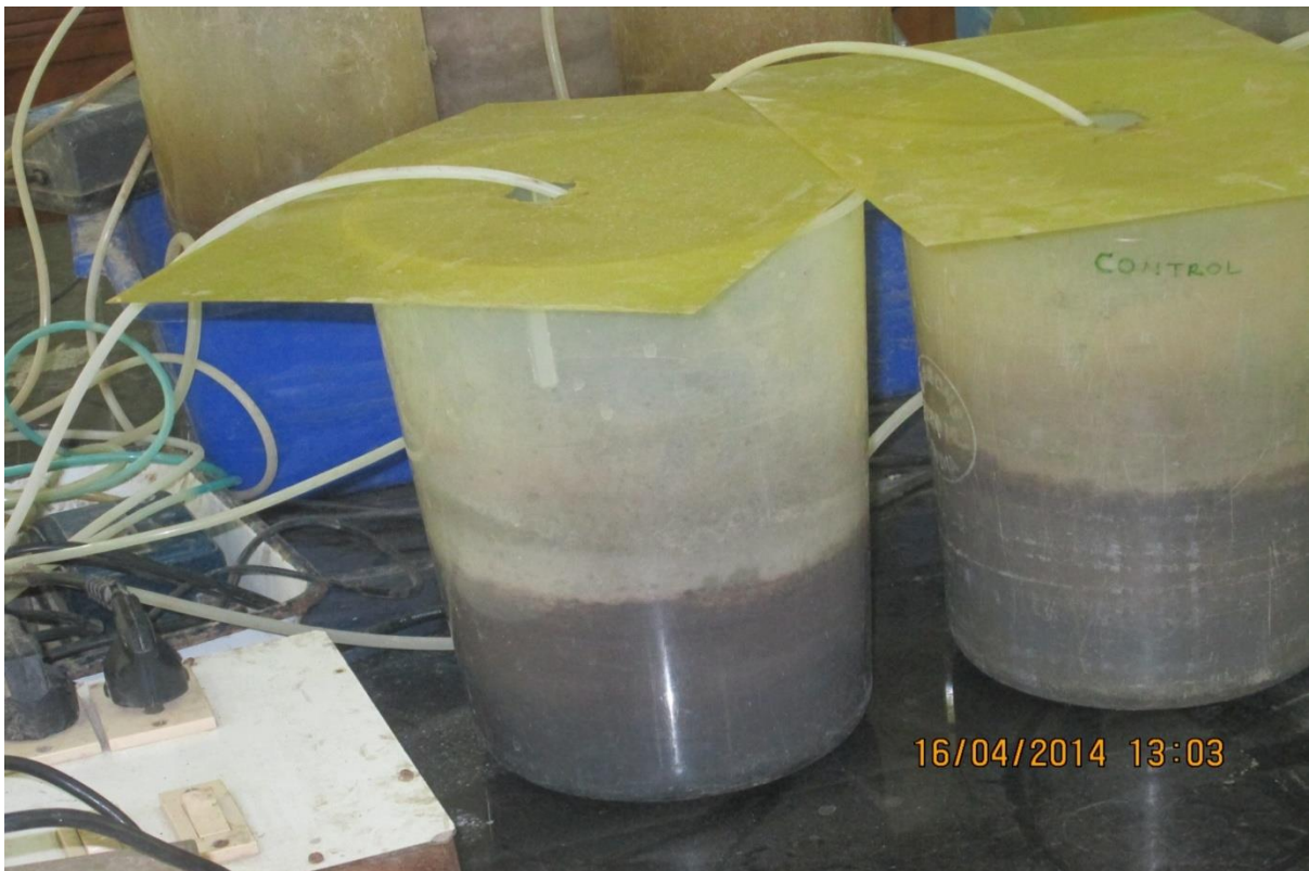
Figure3: SBR reactors for the control and Ozonation
