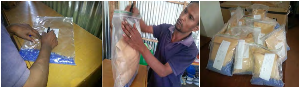
Figure 4.3 Sample handling with self-indicating silica gel at the field
