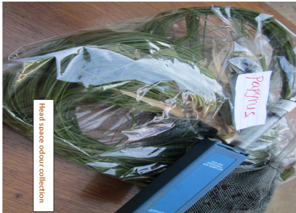
Figure 3.2. Head space grass odour collection using fresh cut grass sample enclosed in a Teflon bag, a Personal Air Sampler with Teflon tubing holding 50 mg Porapak, and a wire gauze bag holding charcoal to filter the air.
