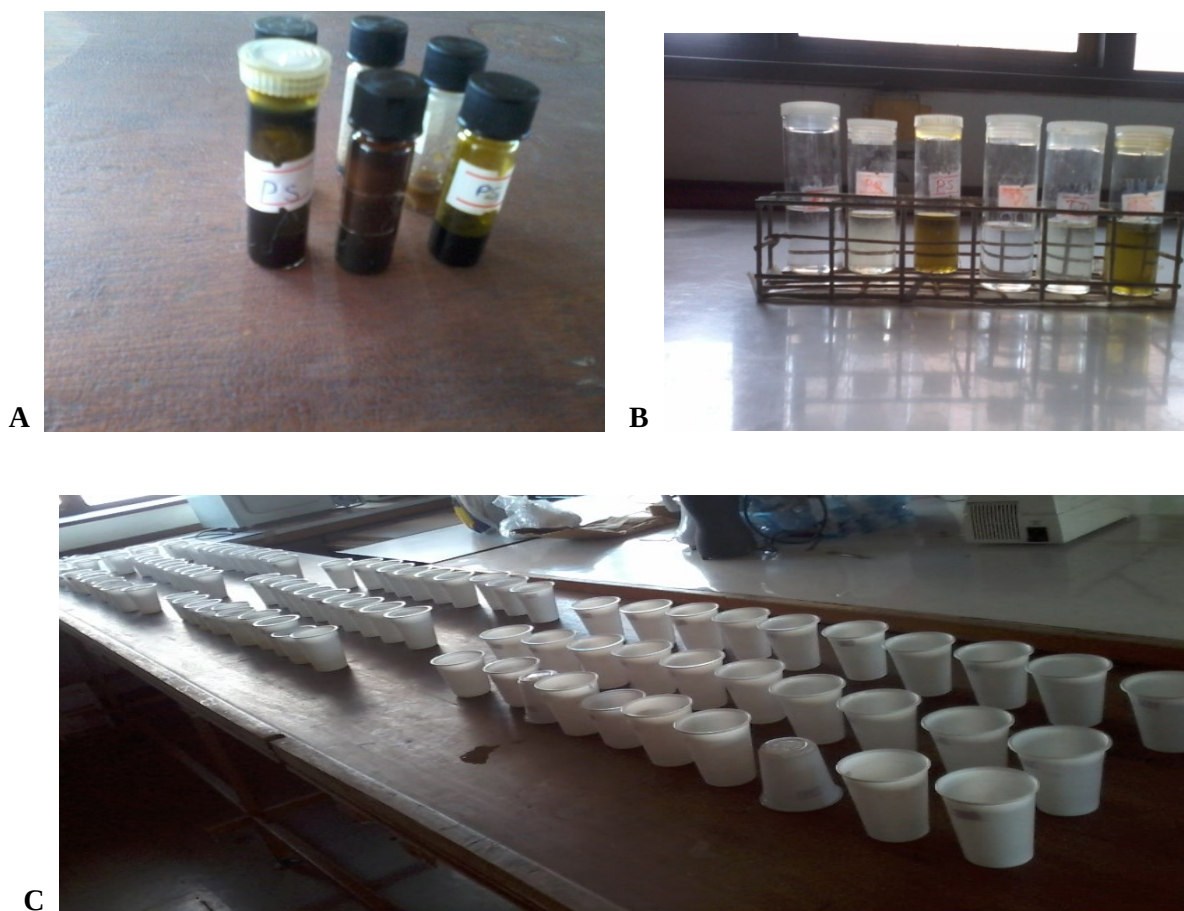
Figure 5.3. Preparation of oils and experiment cups for bioassay procedure: extracted crude oil (A), oils dissolved in solvent ethanol (B), setup of experiment cups (C).
