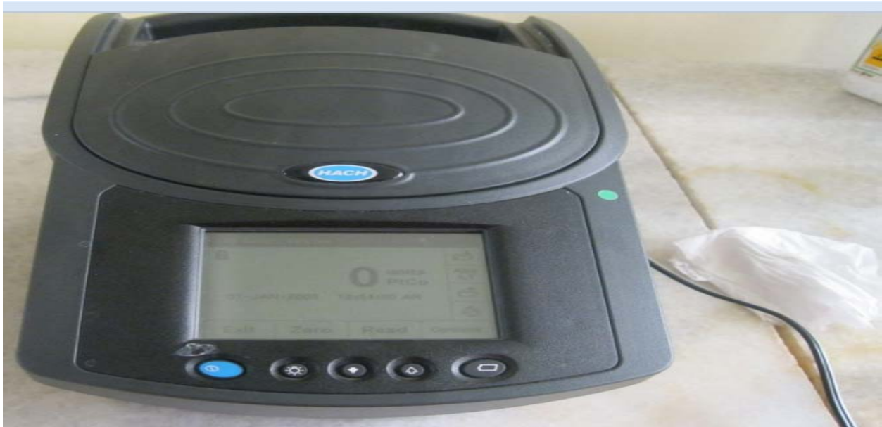
d) HACH DR/2400 spectrophotometer to determine color of K.K waste water
