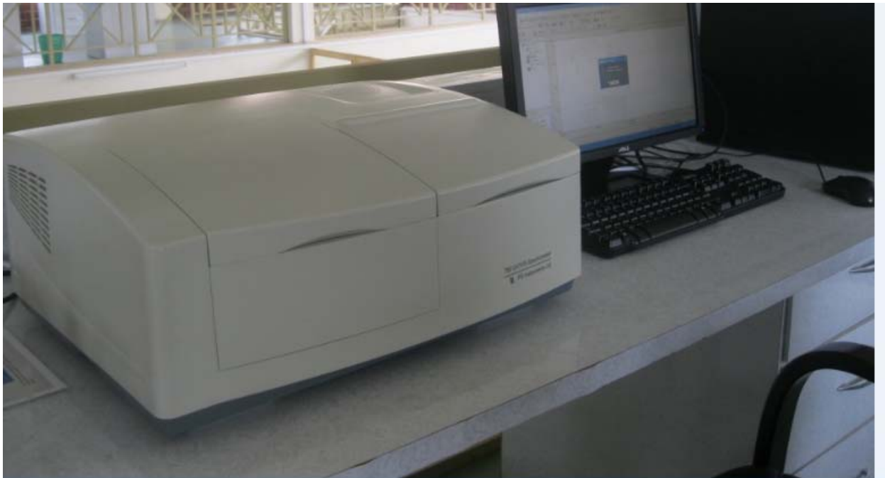
b) UV-VIS Spectrophotometer to determine color of the constituted waste water
