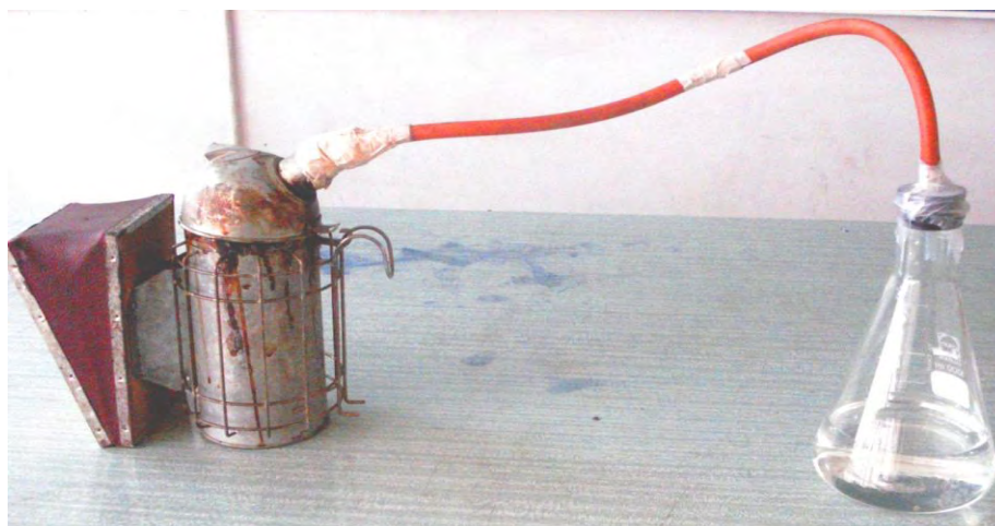
Figure 3. Setup of the bee keeper's smoker for the preparation of plant-derived aqueous smoke extracts.
