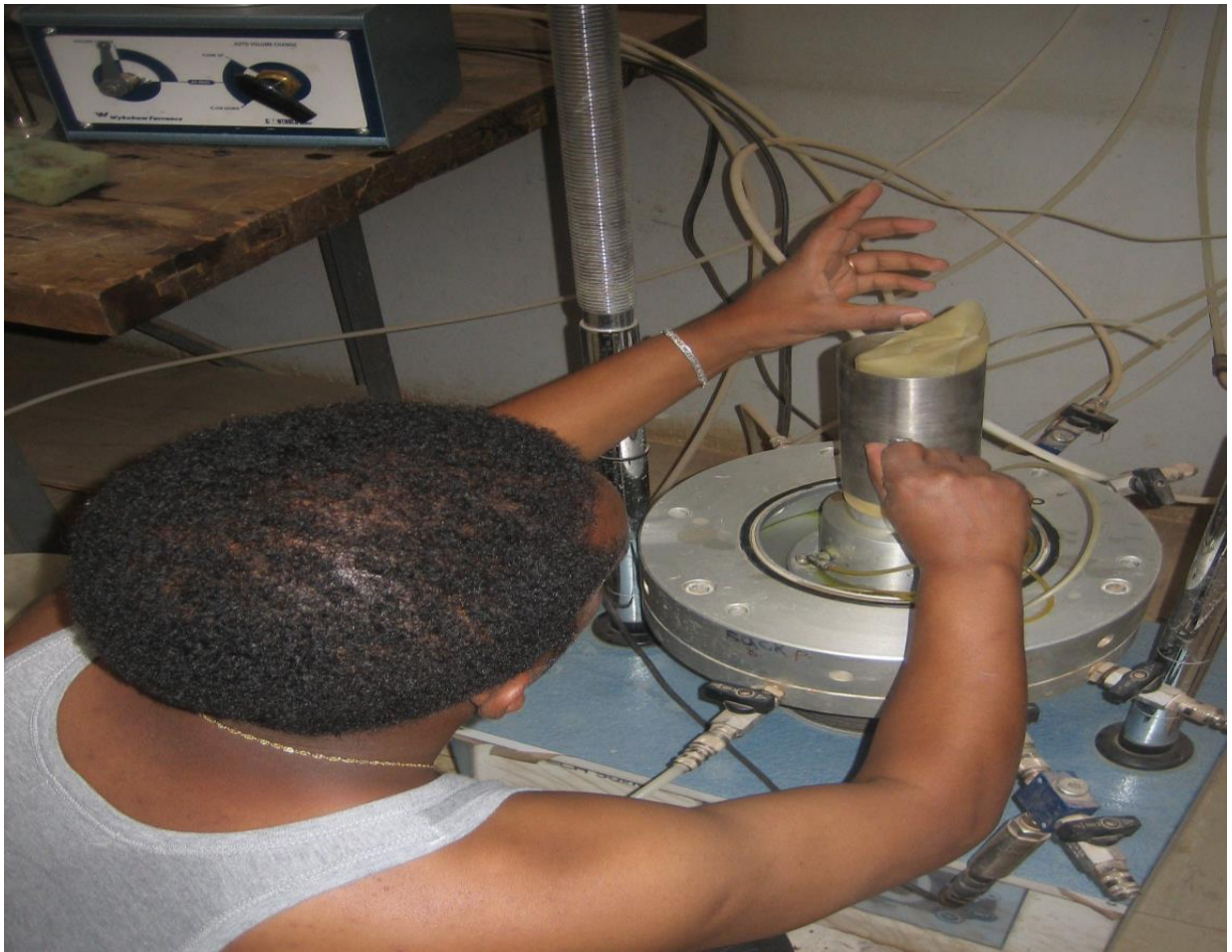
Figure C - 6 Sample being mounted on the triaxial cell
