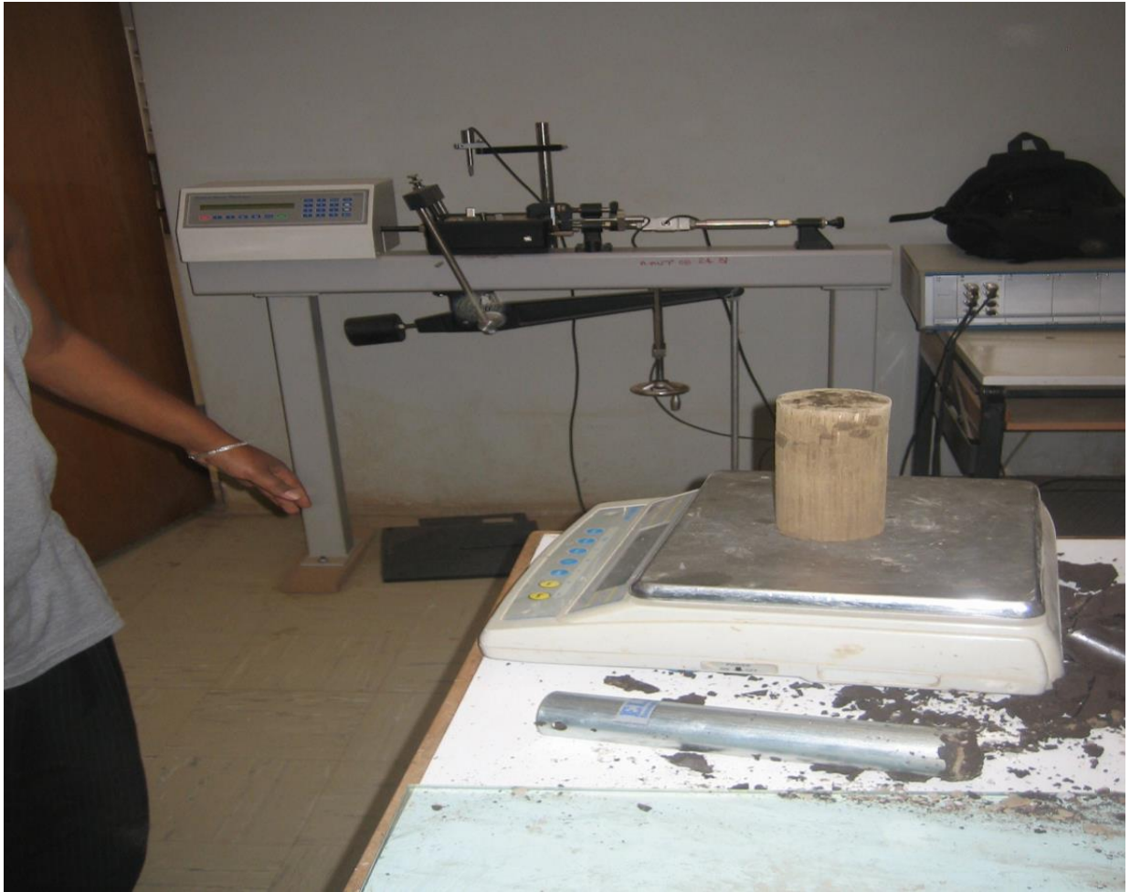
Figure C -5 Sample after extracted from the sampler
