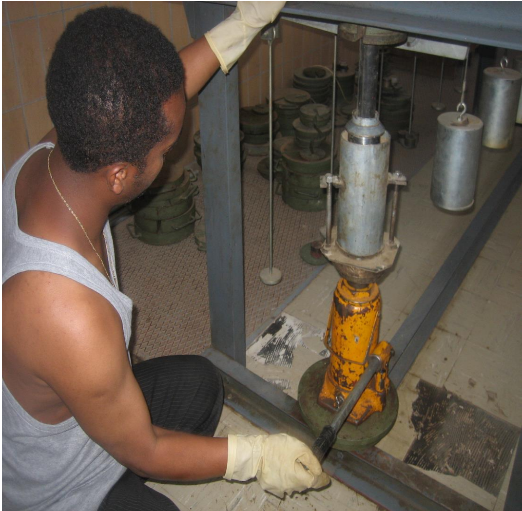
Figure C-2 Inserting the sampler in to the mold
