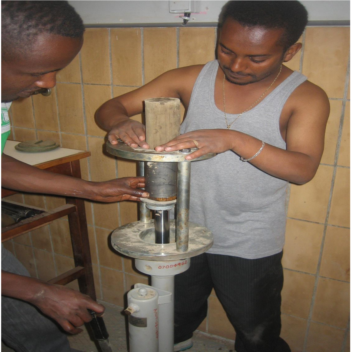
Figure C-4 Extruding the Sample from the sampler
