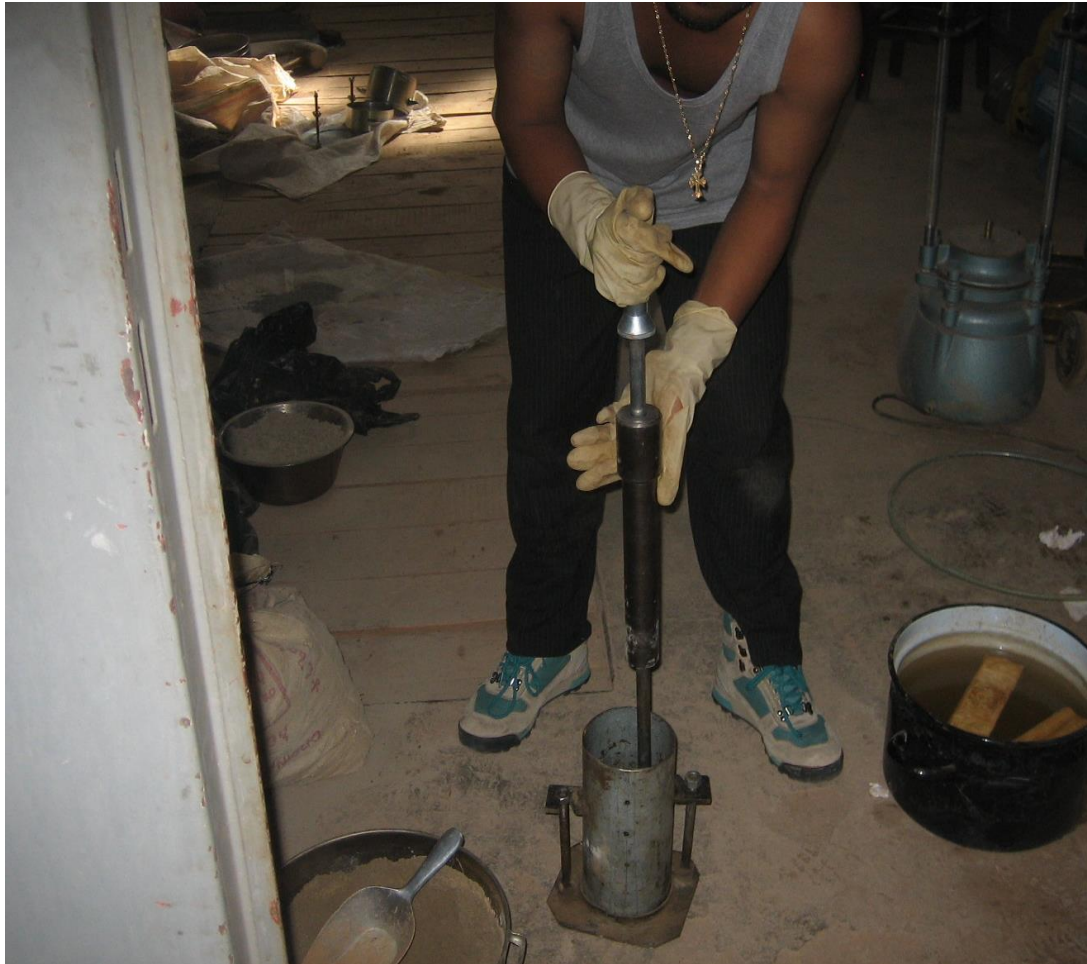
Figure C-1 Compacting the soil in a mold
