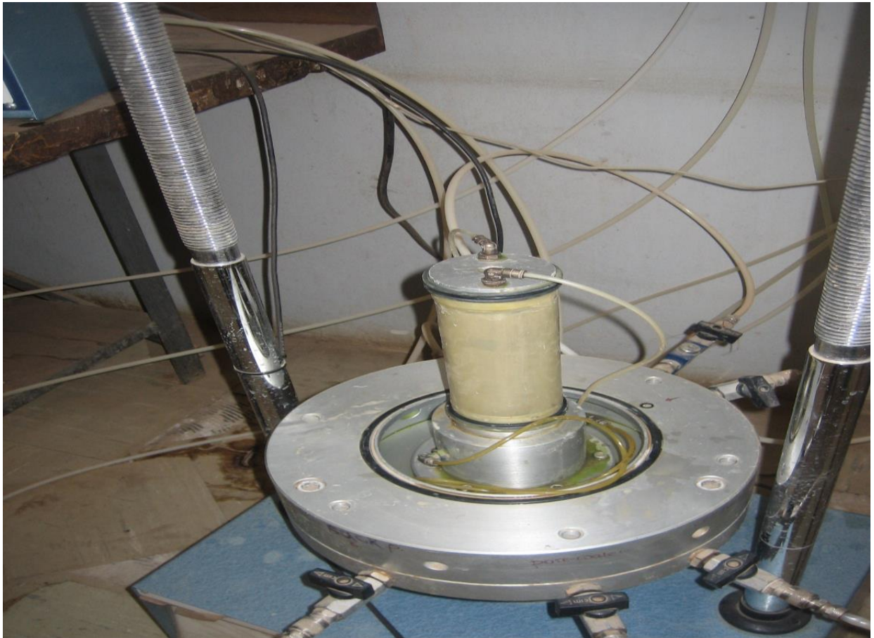
Figure C -7 Sample mounted on the triaxial cell.
