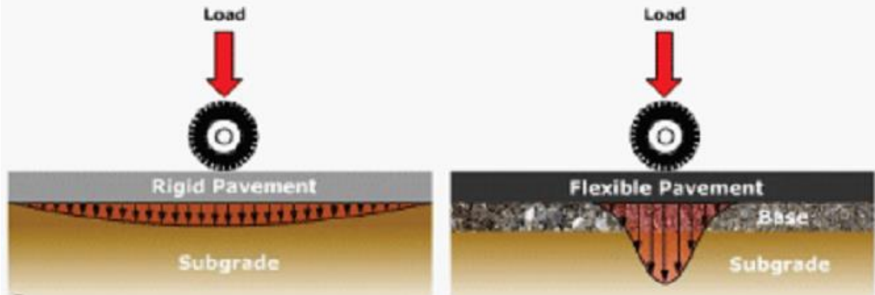
Figure 2: Rigid and flexible pavement load distribution
