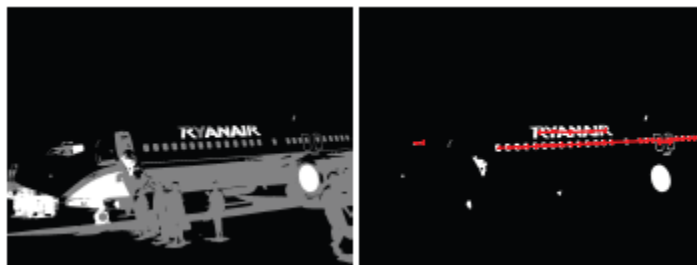
Figure 2. 2 Detected MSER on the left and Letter Candidate on the Right
